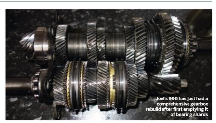
espite planning to sell the car and move on to a 996 Turbo, I have had my gearbox rebuilt, and fitted a brand new clutch and flywheel! To whet your appetite, take a look at the gearbox magnet that Sport and Classic removed – it is literally full to the brim with shards of regurgitated bearings! Next month, you will see in glorious detail exactly what happens when you leave a faint gearbox whining for 20,000 miles!
