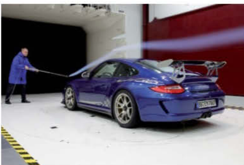
...while the ducktail and huge adjustable rear wing aids downforce at the back of the 450hp Rennsport 997
