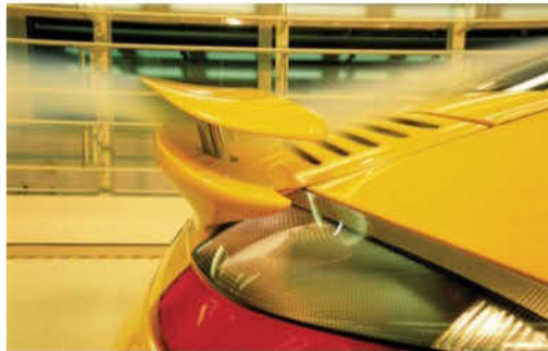
Air flow is analysed on the 996 Turbo's rear wing with PAA
