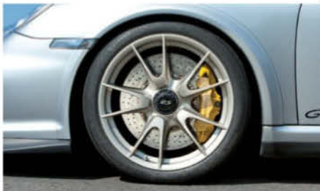
The RS got centre-lock wheels, framing the PCCB brakes and 'Big Yellow' calipers
