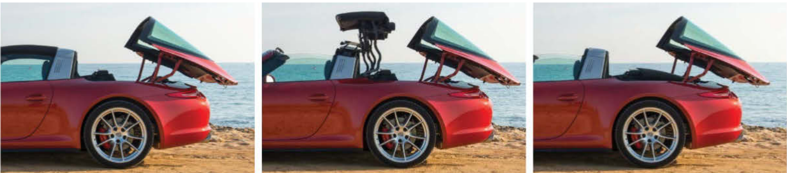
The 991 Targa must be stationary for the roof to operate. Parking sensors in the rear bumper will determine if the glass rear section has enough room to manoeuvre outwards
