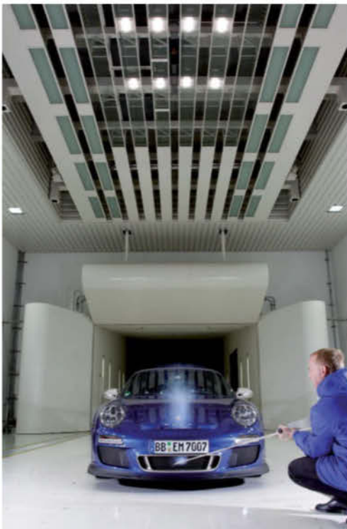
Testing in the wind tunnel helps illustrate the effectiveness of the front air vent's downforce in dispelling air over the top of the GT3 RS...
