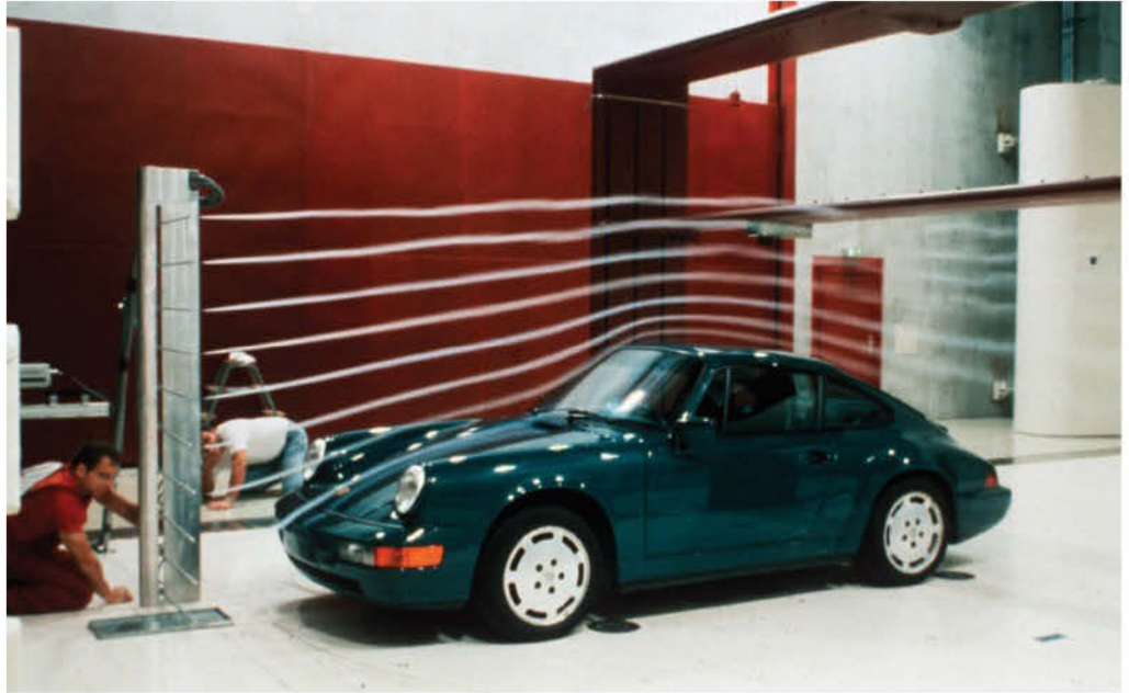
The 964 with substantially revised bodywork over its predecessor goes through aero testing in the wind tunnel in 1987
