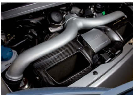
A new intake system, VarioCam Plus and variable geometry turbos contributed to the 530bhp output
