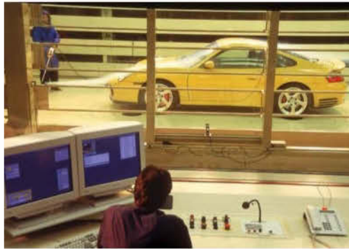
Air flow is analysed on the 996 Turbo's rear wing with PAA
