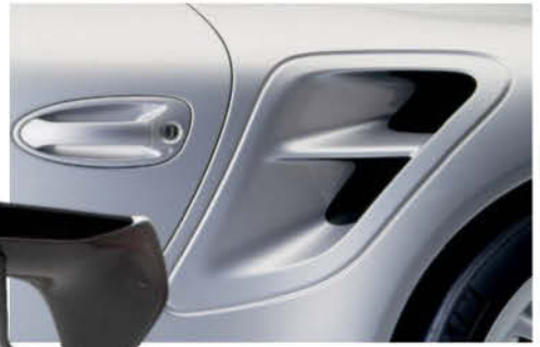
Carried over from the 996, side vents sucked air into the intercoolers at a prodigious rate
