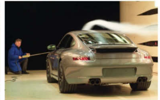
The aero properties of the disguised 997 are tested in '03
