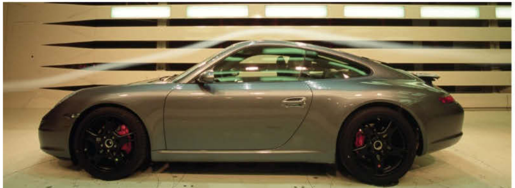
Wind tunnels are essential for understanding the flow of air around a car when in motion. Through the generations, these studies have helped refine the shape of the 911 silhouette to create faster and more efficient models than ever
