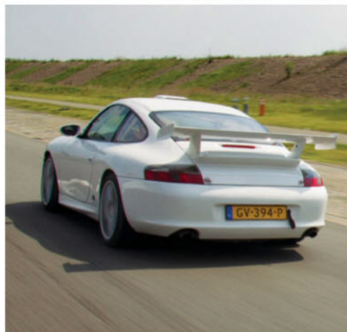
Above Ride height was lifted from 75mm to 100mm and the underside was given a light bitumen coating to protect the car from gravel spray
