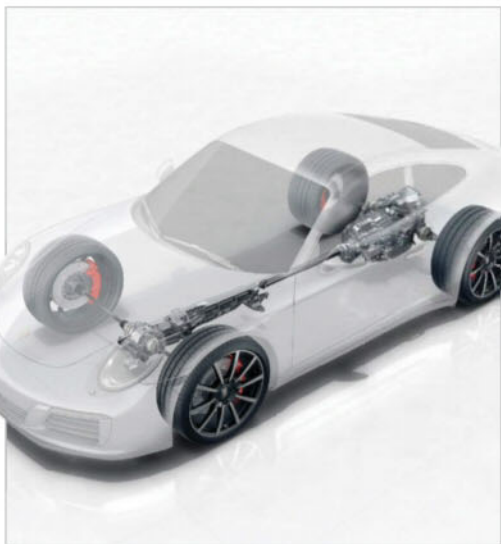
Above Cutaway of the latest Carrera 4's all-wheel-drive system shows how power – and weight – is distributed towards the front axle
