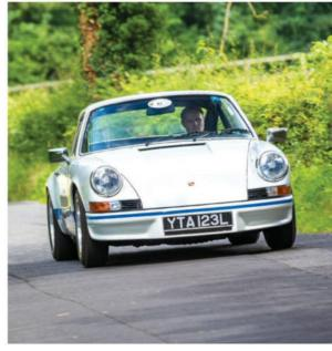
**Left** The 2.7 Carrera RS marked the genesis of the Porsche 911's rear wing with its ducktail. Just 200 2.7 RSs were produced with the M471 'Sport' specification
