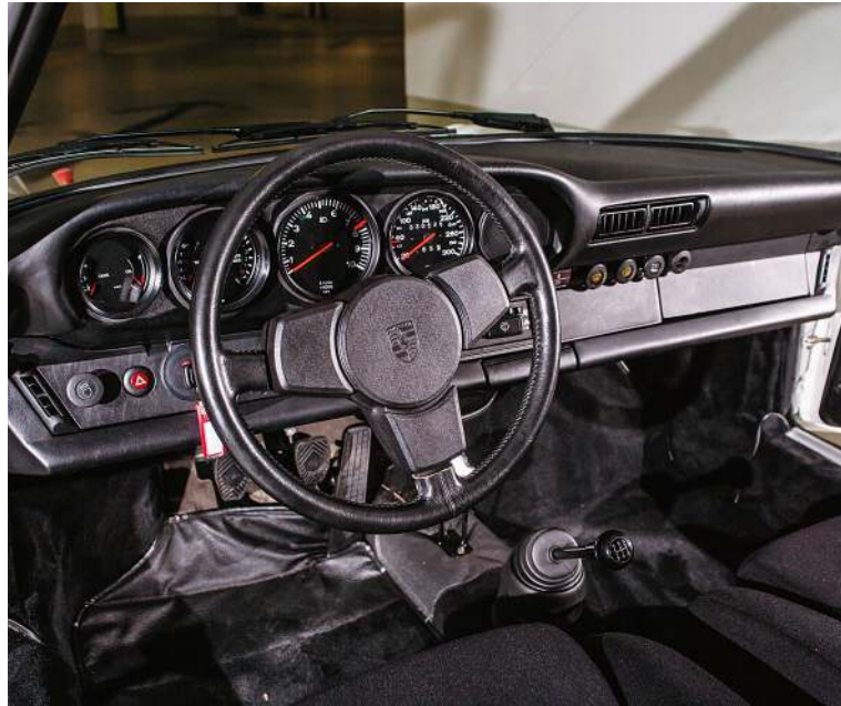
LEFT Note spartan interior with radio and electric window winders deleted. 915 'box is present, as is 7600rpm redline for this rally-spec SC RS
