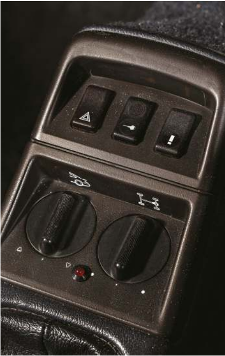
TOP Switchgear for locking differential made its way onto the 964 Carrera 4, but VDO gauge showing torque split remained unique to the 959
