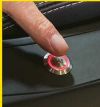
RIGHT KW are keen to educate customers to help them on their journey to improving the handling of their Porsche 911 BELOW Adjustable ride height button is hidden under handbrake lever of KW's 997
