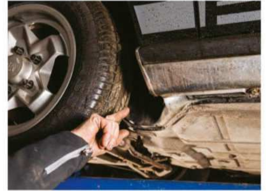
ABOVE Kidney bowls may be the obvious place to look for rust, but a detailed inspection is needed under the whole car
