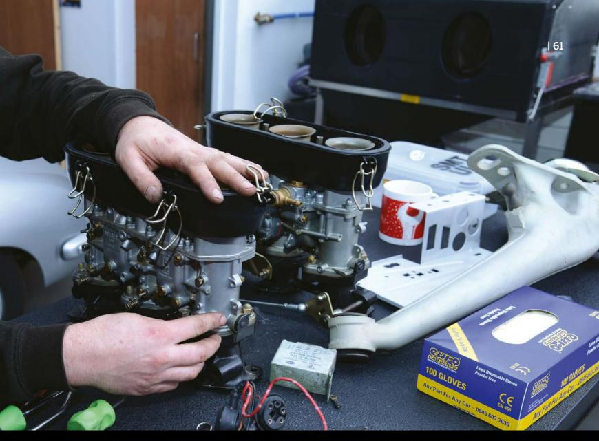
for induction after just 18 months of 91l production, and Weber remained the mainstay until emissions regulations dictated the move to Mechanical Fuel Injection. The Triple Weber system is not unique to Porsche's 91l. The Italian company at that time probably supplied 99 per cent of the performance cars in the world with either single-, double- or triple-choke systems. Triple Webers can be found on Lamborghini, Ferrari and Maserati of the time.
