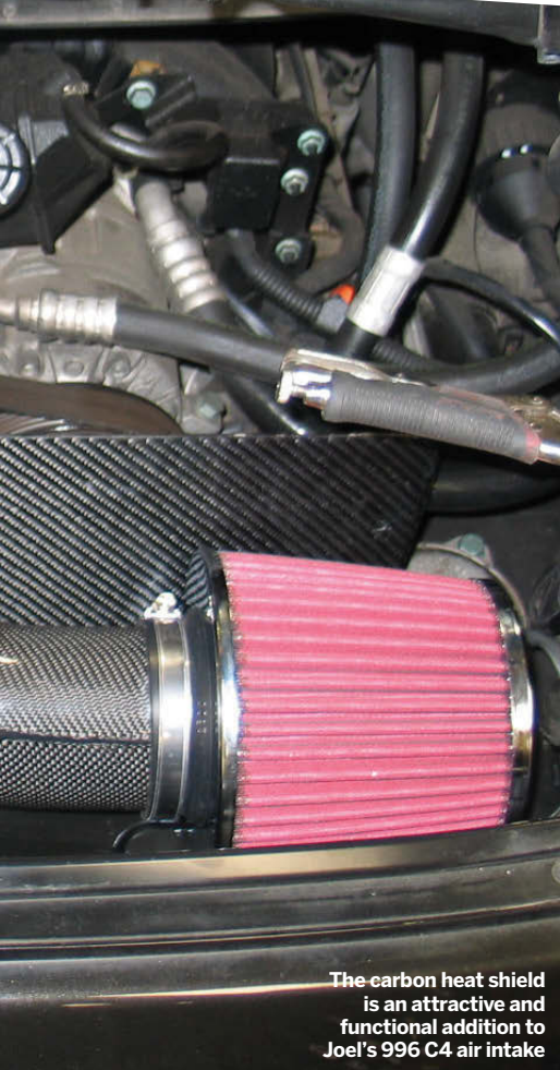
Joel's new induction kit adds to the sound and performance of the car
