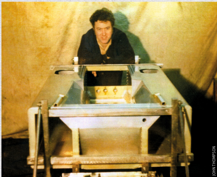
Thompson with monocoque of 312B3. Cortina and roof rack not pictured
