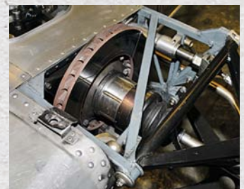
Inboard front brakes were a 72 innovation
