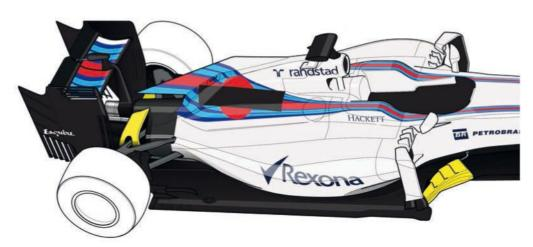
THE WILLIAMS WAS LAUNCHED WITH A NEAT piece of bodywork-shaping at the rear, and the back area also increased in complexity.
