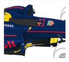
THE AREA UNDER THE RAISED FRONT OF THE chassis is ripe for development. Turning vanes and aero details work with the front wing to create the Y250 vortex, a strong airflow that spirals between the front wheel and chassis to keep the wheel's turbulence from upsetting the car's central bodywork.
