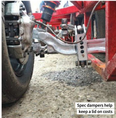
Suspension is fully adjustable
