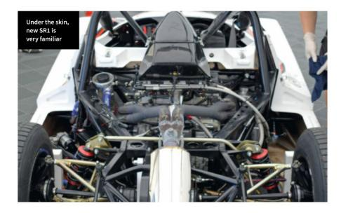
despite retaining almost all its inner workings and capability. Under the bodywork you'll find the same 175bhp RPE (Radical Performance Engines) tuned 134occ Suzuki Hayabusa motorcycle engine and rear-wheel chain drive as the old car.
