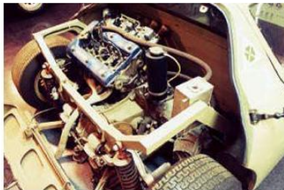
Giulia engine transversely mounted in the OSI Scarabeo.
