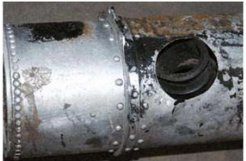
Close-up of the fairly crude arrangement for the fuel tanks.
