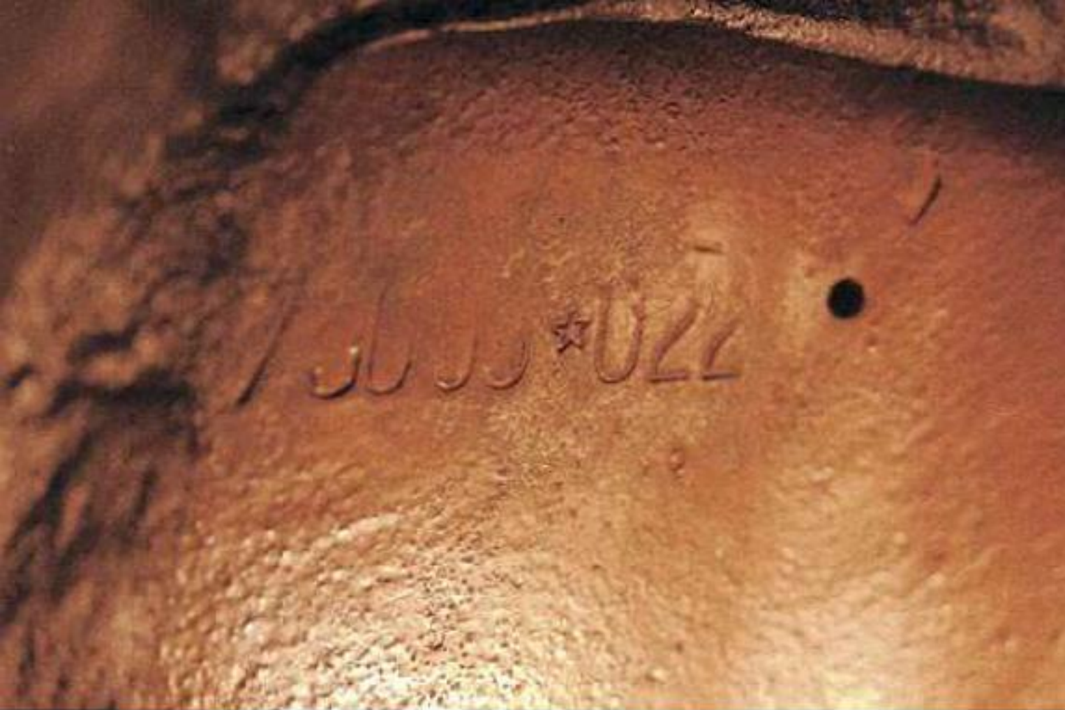
The chassis number stamp on the early chassis tube: 75033.022.
