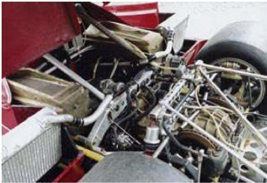
The flat-12 engine is well forward in the tubular chassis.
