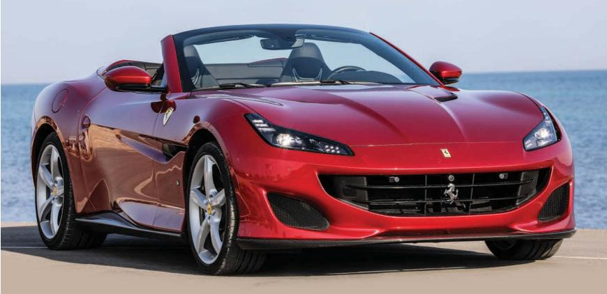
tonneau cover, giving the rear end a 'flow'. New cooling air ducts in the front wings look more purposeful, while a front end design described as "grintoso" (gritty) gives it extra aggression. The aerodynamics are improved, too, by six per cent (Cd 0.312).
