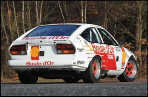
compression to the rear. This means that the braking effort can be better shared fore and aft, hence the large rear brakes. Braking is a strong point with lan's Group A car. Together with slick tyres, lan's car might manage a deceleration of 1.4 g compared with 1.2g for the Group 2 and 1g for the Group 1b. Lateral-g (cornering forces) would be in a similar ballpark.
