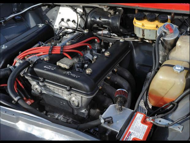
2.0-litre engine makes for strong performance. Lower roll centre with rear end mods sharpens up handling
