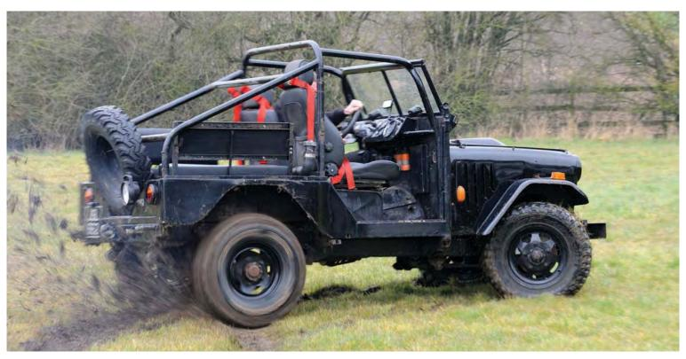
absorbers which significantly improve the ride and off-road ability. A hydraulic diff locks front and rear instead of cable operated ones found on a standard Matta. Alfa 156 leather front seats and a set of rear bench seats from a Land Rover have been fitted for ease of cleaning when it gets really muddy
