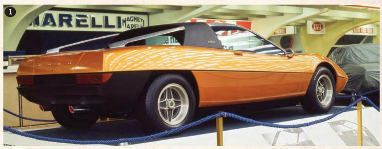
**01.** Ford's GT70 was constructed with rallying in mind. Ercole Spada of Ghia was tasked with shaping the production version which would have featured a Cosworth BDA four or Ford Cologne V6 power, but the car pictured here remained a full-scale model. Just to add to the confusion, the design has also been attributed to Filippo Sapiro...
