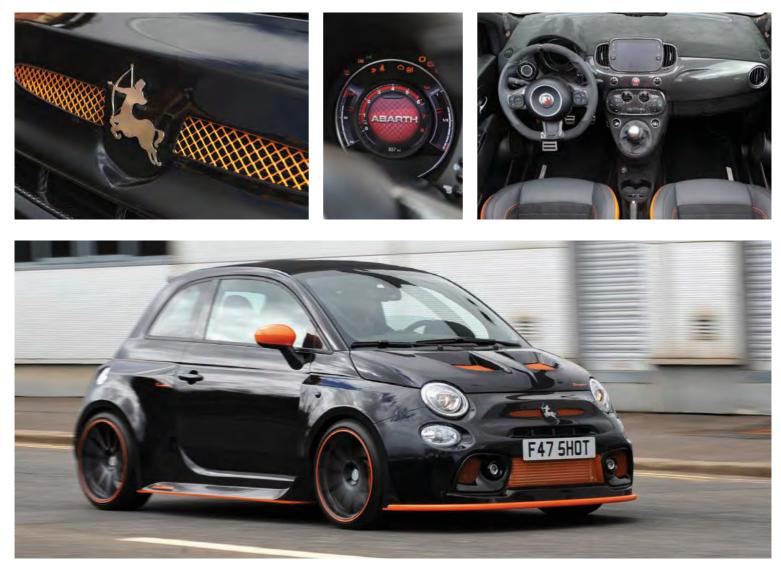
Big front end has function as well as fury, allowing air to flow into the frontmounted intercooler large front-mounted intercooler which feeds a whopping custom hybrid turbo.
