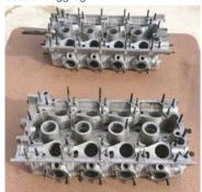
Ferrari 308 cylinder heads. Ferrari 308 V-8 cylinder heads, 2 valve design from mid to late 70's, part # 105939 (left) and # 103514 (right). Good used condition, rebuildable, minor scarring on intake manifold surfaces from disassembly. These are US market heads with air injection into exhaust ports, air injection manifolds included, \$1800. Email: clance840@gmail.com. A253/065
