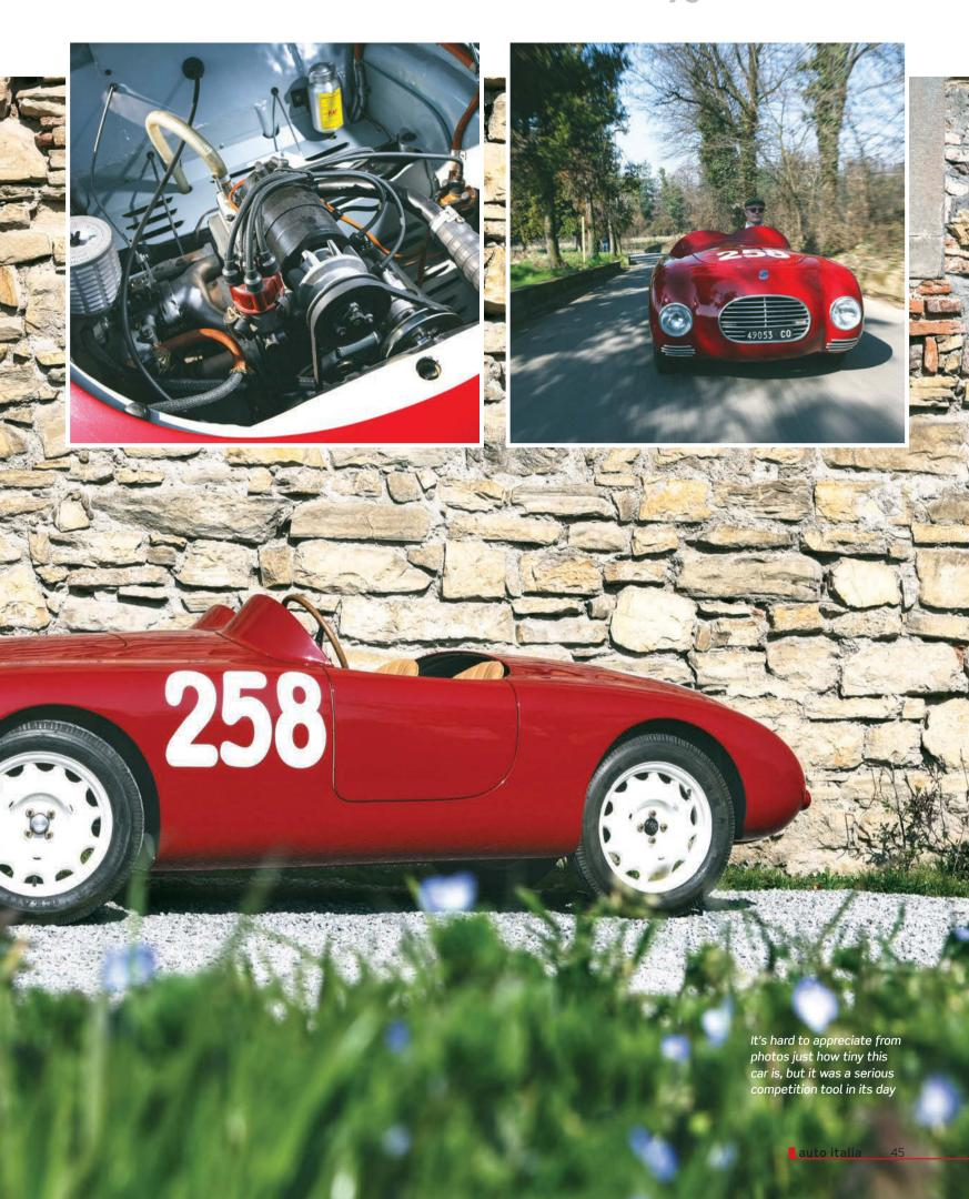
work of brothers Mario and Domenico Fenocchio of Brescia. Based on a regular Topolino chassis, but featuring a full-house 742cc Siata-headed Fiat 'four', the body was created by Carrozzeria Bresciana. Unusually, it was formed from steel, with the bonnet and doors in aluminium.
