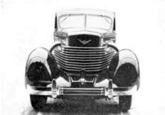
Head-on view of a 'one-off' extra-long wheelbase, six-window limousine. Note added height of hood requiring lengthened outside exhaust stacks and ten louvres!
