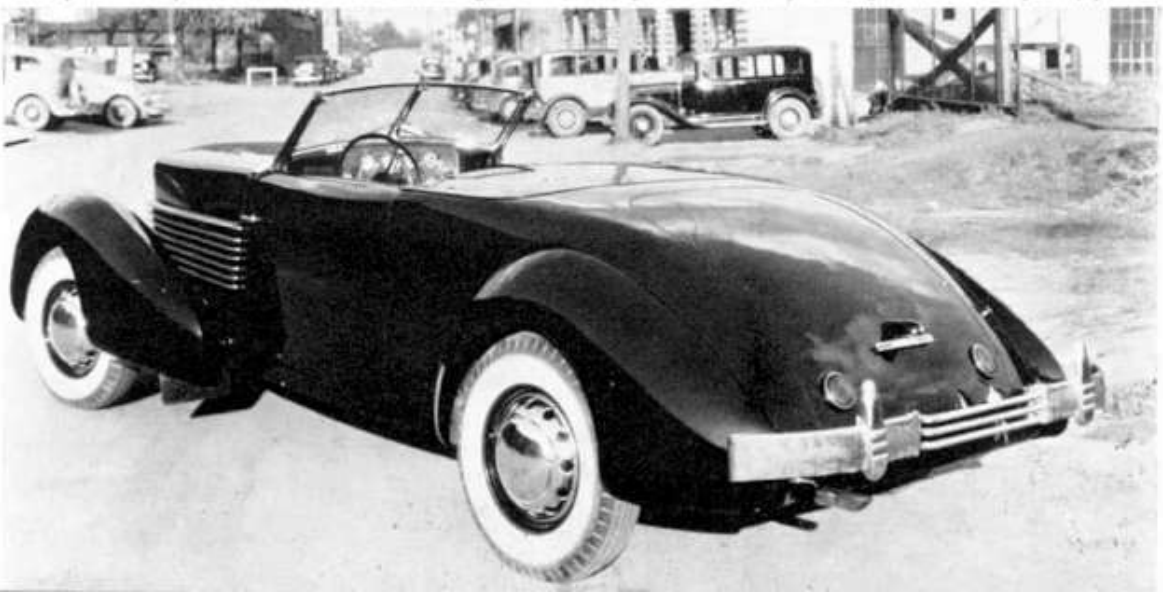
An early Model 810 Sportsman as it comes off the line. The completely hidden folded top contributes immeasurably to the sleek, good looks of this beautiful convertible. Protective covering on chrome bumpers dulls some of the brightwork in these factory photos.
