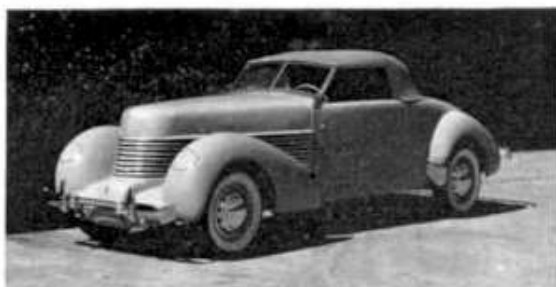
A 'mock-up' Sportsman, perhaps a prototype for a 1938 or 1939 model, shows 8 louvres in a downward and progressively forward protruding modification of hood (bonnet) styling. A simplified rounded and higher transmission cover replaces the 'wrap-around' configuration of the original housing.
