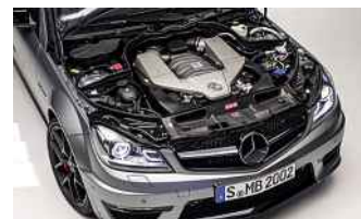
Above: piston and crank upgrades have boosted the C63's 6.2-litre V8 to 500bhp
