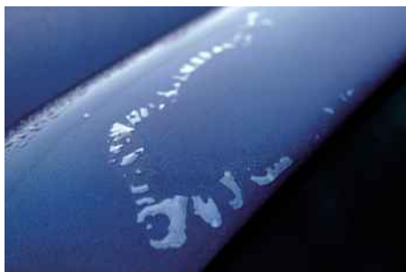
Above: paint is starting to flake off the Clio's rear spoiler, and one of its gold-painted alloys needs tidying up too
