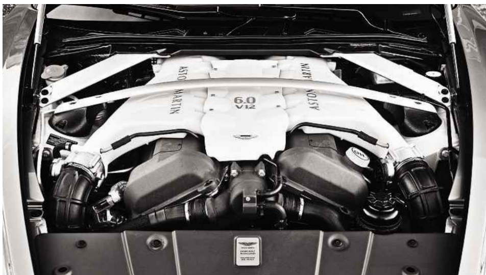
Above: huge 5935cc V12 is shoehorned into a tightly packed engine bay. Opposite page: Zagato gets unique trim
