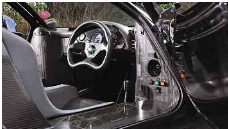
Above: XJR-15 carries true racing looks. Below left: cockpit is trimmed simply in carbon and Kevlar; wide sill makes entry and exit tricky. Below middle: just 50 road cars were built
