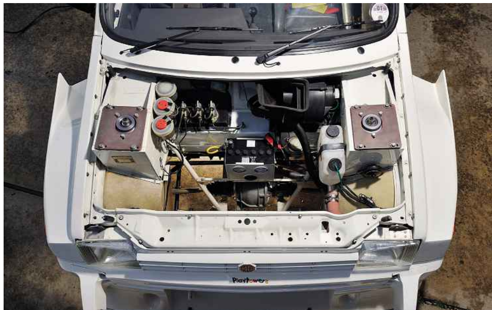
Above: with the 3-litre V6 in the back, the front of the 6R4 houses little more than driveshafts and the front diff
