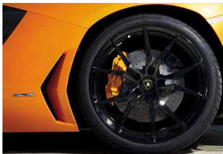
Above: removing the roof adds a new dimension to the Aventador. Right: huge 400mm carbon-ceramic discs sit behind the front wheels; LHD cars have better pedal position; 6.5 V12 sits beneath glass panels
