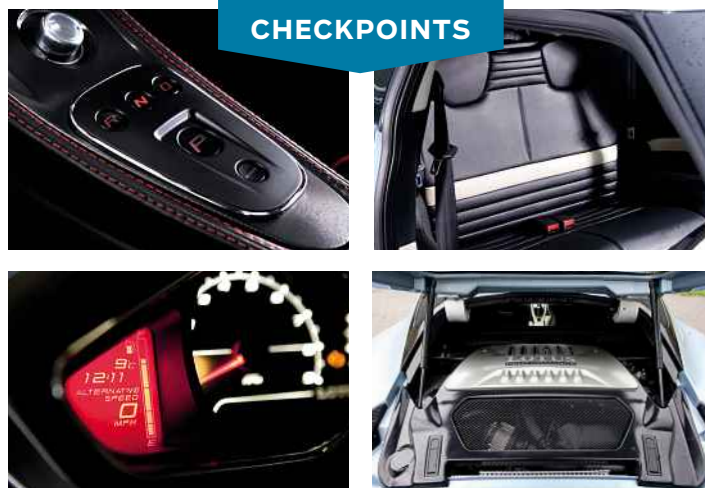
Clockwise from top left: 'Intelligent Precision Shift' auto is a torque converter; optional rear seats are of limited use; Toyota engine reliable; expect 25-30mpg
