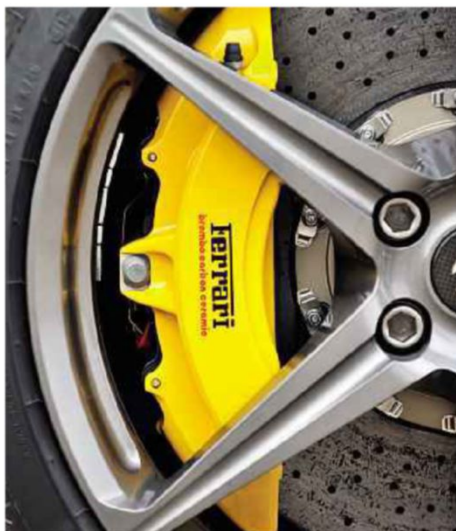
Above: 458 has carbon-ceramic discs as standard; the 398mm fronts are larger than the R8's and MP4-12C's
