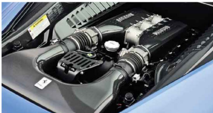
From left: Audi V10 engine is the largest of the three by capacity (5204cc), but at 542bhp is the least powerful; Trott's McLaren long-termer carries the latest engine upgrade to 616bhp; Ferrari's 4.5-litre V8 hits 562bhp peak at scorching 9000rpm
