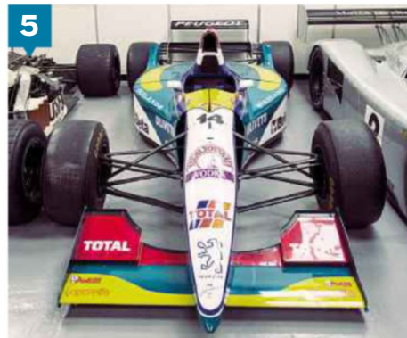
Above: 1995 Jordan F1 car, as driven by Rubens Barrichello; engine is a 3-litre Peugeot V10
