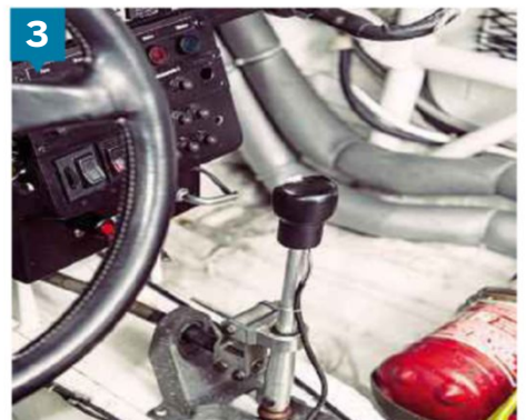
3 Above: button atop the Audi Quattro S1's gearlever automatically dips the clutch on changing gear
