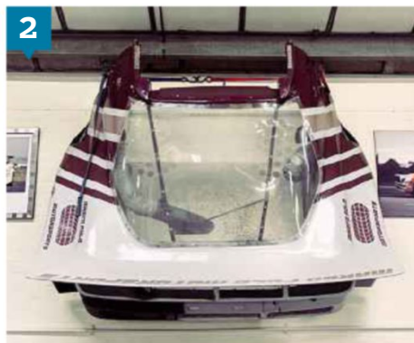
2 Above: IMSA Ford RS200 rear clamshell – complete with near-vertical spoiler – hangs on the workshop wall
