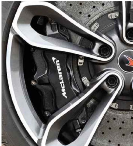
Above: this MP4-12C runs optional carbon-ceramic brakes; 305-section rear tyres are the widest here
