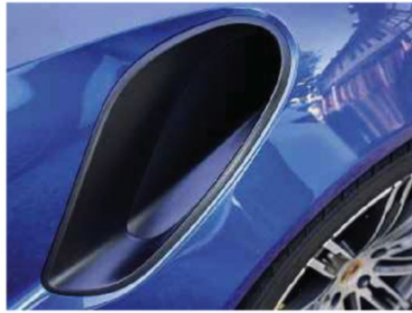
Left: huge intakes feed the 3.8-litre twin-turbo engine; as before, the turbos have variable-turbine geometry. Below: Turbo S revs all the way to 7200rpm
