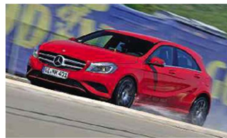
Top and above: straight-line aquaplaning test looks for slip levels greater than 15 per cent on one wheel
