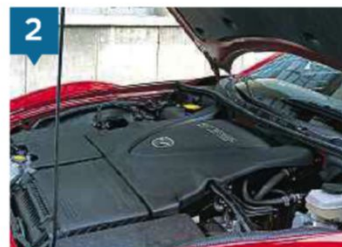
1: RX-8 enjoys sweet handling balance, but fuel economy is poor. 2: keeping Wankel rotary topped up with oil is crucial. 3: most interiors are still in good nick
