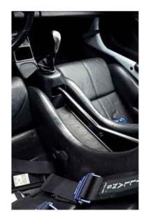
Right: gear linkage runs exposed between the two seats. Below: 1996 and '97 cars were lefthand drive: '98 machines were RHD to help drivers on circuits that ran mostly clockwise. Bottom: the later '97 and '98 GT1s, in silver and white respectively
