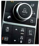
Above: Hybrid version returns 44.1mpg on the combined cycle. Left: EV mode (bottom-left button) allows for a mile of electriconly driving
