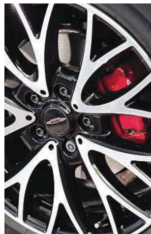
Above, middle: big central speedo still dominates Mini cabin. Above: Paceman is over 50bhp down on its rivals here – and it shows. Left: Mini's 307mm discs are the smallest front rotors in our group
