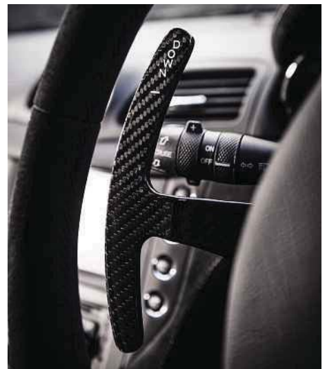
Above: single-clutch paddle-shift in the MC Stradale lags behind in shift times. Right: both cars run Brembo carbon-ceramic brake systems
