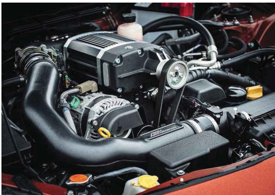
Right: supercharger sits exposed on top of the flat-four. Below right: new multi-function gauge sits in air vent
