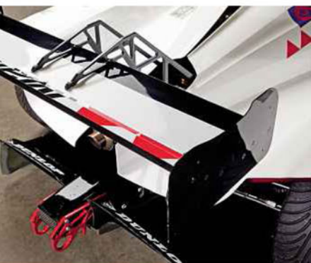
Above: Catchpole acquaints himself with overhead buttons. Below: rear wing contributes to over 600kg of downforce. Right: 210bhp 2-litre engine is sourced from Formula Renault racer
