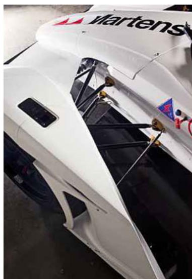
Left: cabin looks dark and cramped, but outward visibility is good; exposed wishbones ape single-seater design. Below: Dunlop race tyres are fitted, with wets (pictured) and slicks available to suit the conditions
