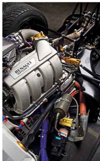
Above: Catchpole acquaints himself with overhead buttons. Below: rear wing contributes to over 600kg of downforce. Right: 210bhp 2-litre engine is sourced from Formula Renault racer
