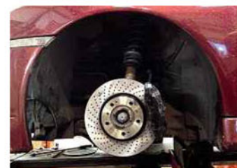
Above: rather than getting a full brake system upgrade, Bovingdon limited himself to Eurocup GT discs (right) and EBC Yellowstuff pads (below)
