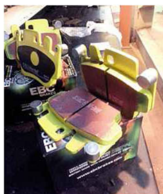
Above: rather than getting a full brake system upgrade, Bovingdon limited himself to Eurocup GT discs (right) and EBC Yellowstuff pads (below)
