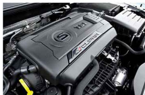
Above left: four-cylinder turbocharged engine gets 276bhp in '280' trim. Above right: flag badges are amongst the relatively subtle Cupra styling cues. Below: Alcantara seats are standard; full-leather is an option
