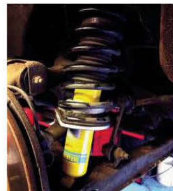
Left: back in the workshop, this time to have Bilstein dampers (above) fitted. Below: Bilsteins work well with Eibach springs previously installed. Bottom: yellow Bilsteins just visible
