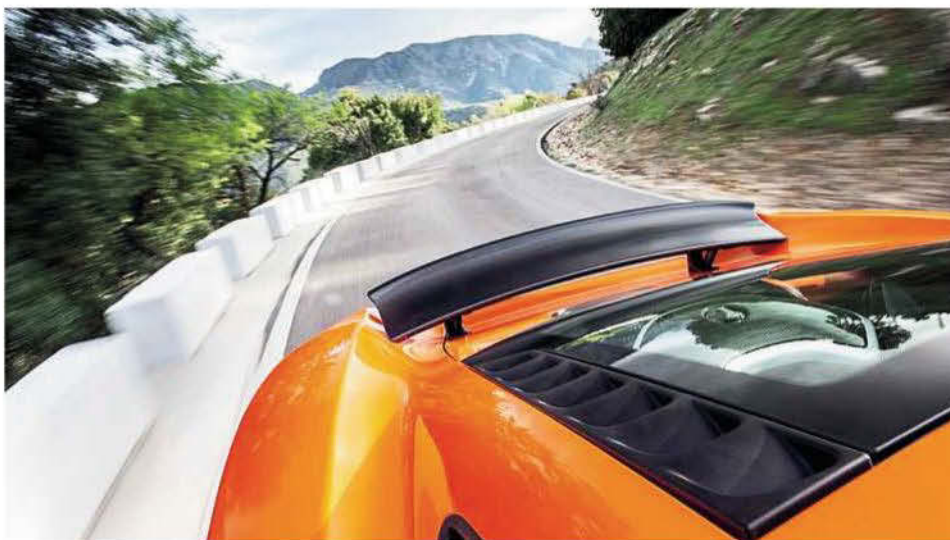
Above: Airbrake deploys to improve stability when lifting off or cresting a hill; this new functionality, along with a DRS mode, will be offered to existing 12C customers as a free 'Technology Upgrade'
