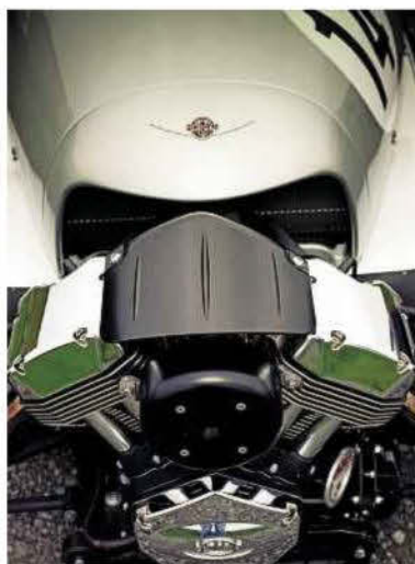
Right: 2-litre V-twin sits at very front of Morgan. Below: pair of centre console buttons operate heated seats(!). Bottom: modern double-wishbone front suspension supersedes Morgan's sliding pillar technology of old
