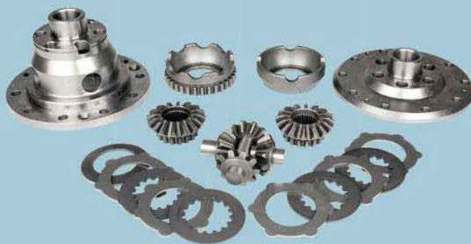
Above: Torsen diffs are only fully effective when both wheels are on the road. Below: what you'll find inside a clutch-based LSD
