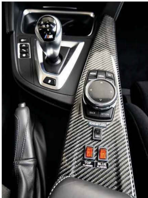
Above: switches to operate safety lights are additions to carbon centre console. Below: rear seats make way for half-cage and fire extinguisher
