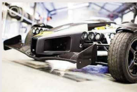
Left: optional sidepods aid cooling; wing increases front grip. Below: Atom's 'naked' look remains its hallmark
