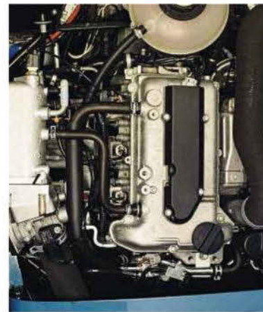
Opposite page (from top): narrow Long Mynd road is ideal for such diminutive sports cars; Catchpole finds rewards from keeping the Caterham's narrow tyres at their limits. Left: 660cc turbo engine is fitted with room to spare. Below: short-throw manual lacks a little precision. Bottom: double-wishbone front suspension is exposed
