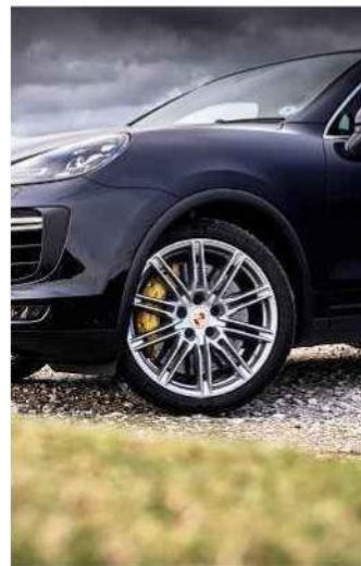
Top: SVR isn't naturally agile, and often needs to be massaged through corners. Left: £5924 carbon-ceramics aim to improve handling on the Cayenne by reducing unsprung weight. Below: X6 M has the best steering feel in this group
