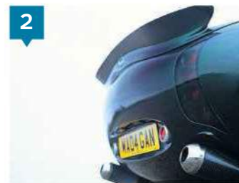
1: Mk2 Tuscan gained faired-in headlights... 2: ...and tail lights gathered together in clusters (rather than individual lights in various positions on the rear). 3: interior remained bonkers
