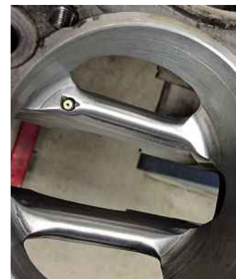
Above: the cylinder case before (left) and after the webs were 'boat-tailed' for smoother air movement
