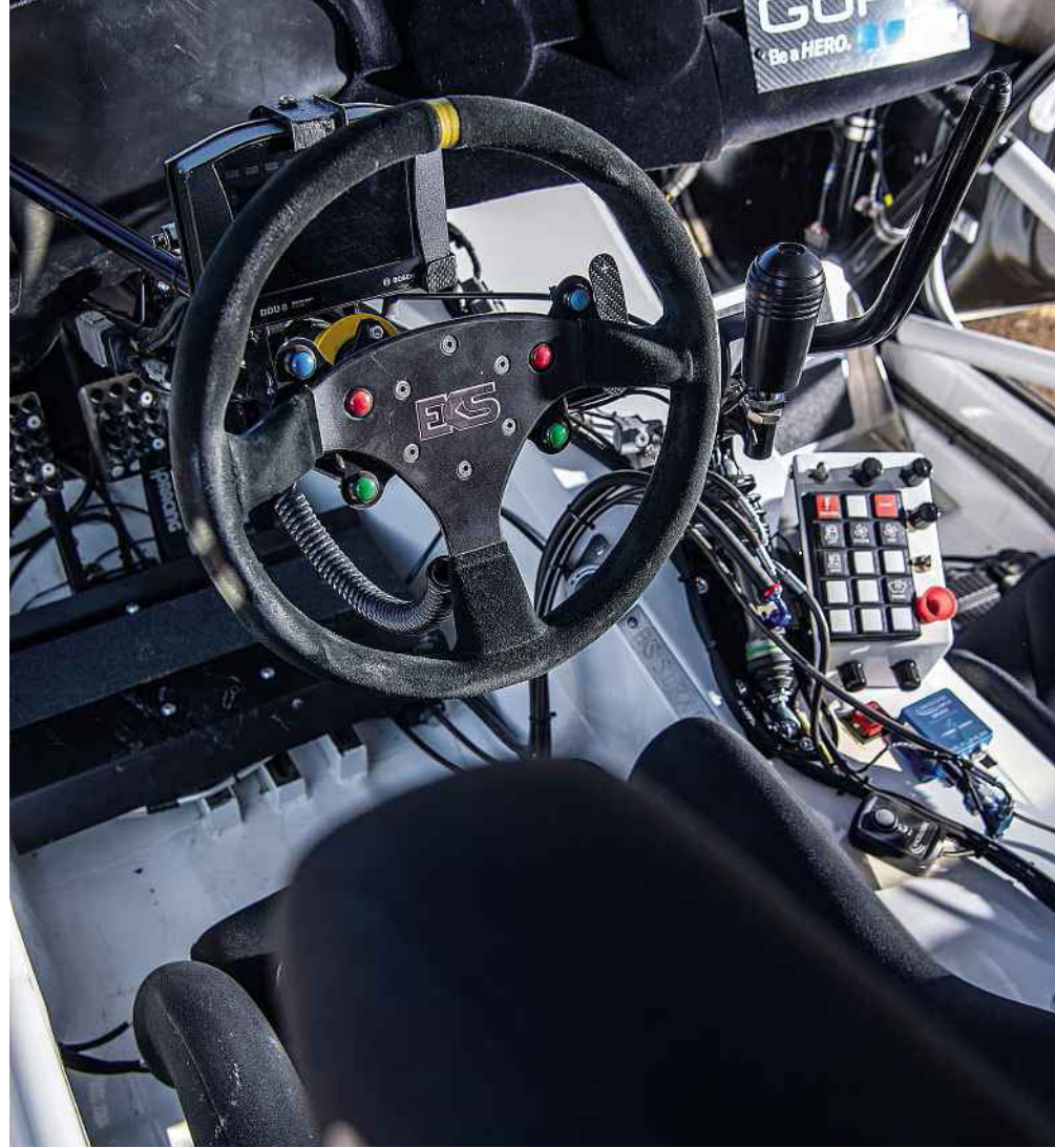
Above left: enormous handbrake disconnects drive to the rear wheels, allowing the driver to lock the brakes. Above: press blue for anti-lag. Left: transversely mounted turbocharged 2-litre engine develops around 565bhp
