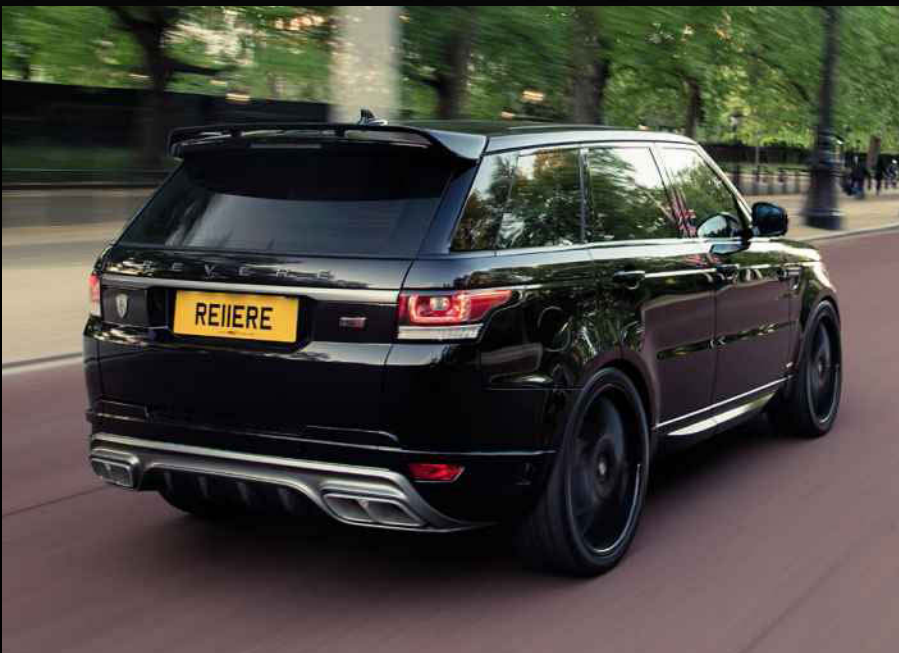
Rear Bumper featuring Solid Billet Aluminium Exhaust Tailpipes and high-level Boot Spoiler
