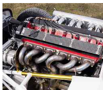
Top: superformed aluminium bodywork sits over a tubular steel chassis. Above: 4.2-litre straight-six is rebuilt using new components
