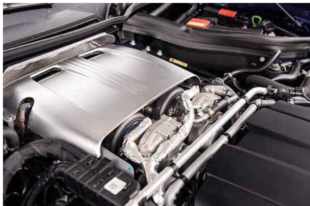
Above: twin-turbo V8 sits well back in the AMG's engine bay, aiding the car's balance. Below: beneath all the luxury-tourer garb the AMG GT is a proper sports car
