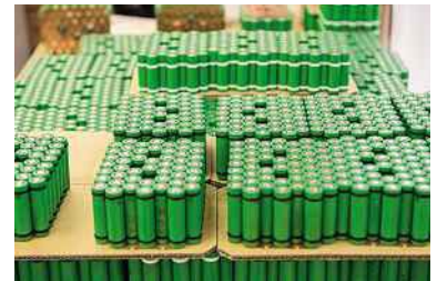
Above: battery cells – lots of them – waiting to find a home in the Concept One's T-shaped power pack.
