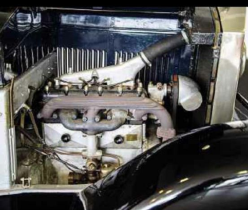
Above: Harry Ricardo's first car engine – from a 1930s Citroën Rosalie.
