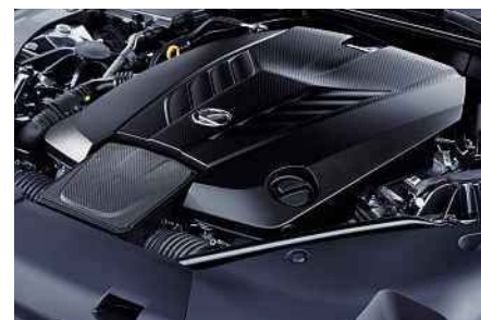
Above: interior is beautifully finished but has some clumsy details – witness the controls protruding from the instrument binnacle. Right: main attraction is the 5-litre, 470bhp, naturally aspirated V8, which just loves to rev
