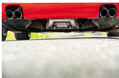
Top: red line isn't till 8500rpm, and engine doesn't really come alive until the needle passes 6000rpm. Above: F355 was one of the first road cars to use underbody aero to create downforce
