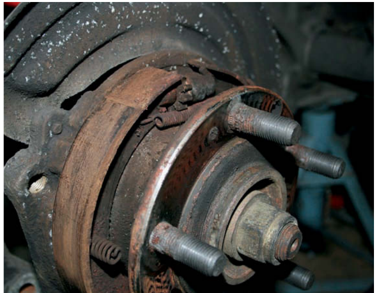
Matt has been grappling (quite literally) with a broken handbrake on the 924, which has required some minor surgery on the brake system
