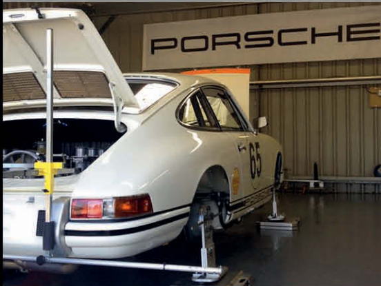
SUSPENSION REBUILDS AND SET UP
