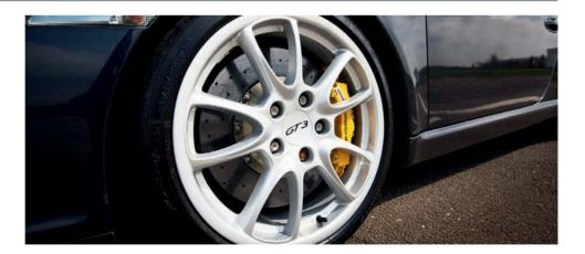
UK firm Surface Transforms have partnered to develop a Carbon Ceramic brake kit available for Porsche applications in three formats. The first is as direct replacements for OE components, for greater strength and significantly higher thermal conductivity for improved driveability, and more consistent performance on the limit.
