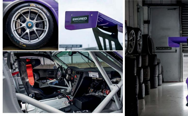
A weld-in roll-cage dominates and there's also an integrated system for fast driver extraction in the event of an accident
