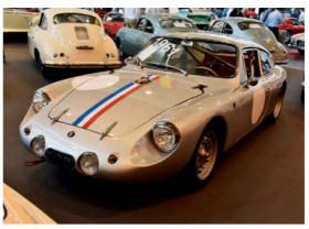
This is a 1961 APAL Porsche Coupé. Just 150 were made between '61-'65, 30 of which (including this one) used 1600cc (95hp) Porsche 356 (Type 616/7) engines, gearboxes, wheels, brakes and instruments
