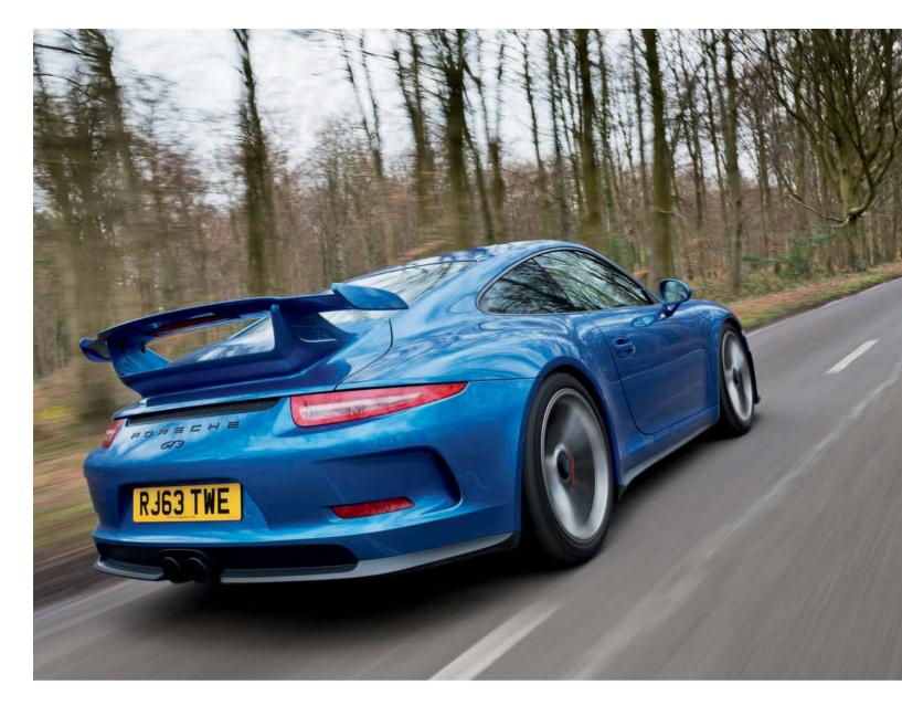
Gen 2 GT3 debuted lightweight (3kg lighter than the Gen 1 versions) alloy wheels that, along with lighter springs, served to reduce the car's unsprung weight. Tweaks to the PASM system meant ride comfort was improved even further while changes to the car's roll bars resulted in a stiffened chassis capable of quicker turn-in and reduced understeer.
