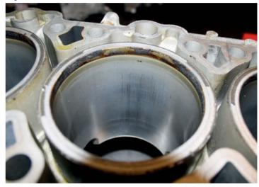
cases are the Tiptronics between 20-40k miles. They never go through the correct heat cycles, are always used for short journeys at low revs, with the fuel washing the bores. The 3.8s are slightly worse, but we see the 3.6 and sometimes the 3.4 Cayman S engines as well. When these cars come in for their two-year service, the oil is like black treacle and you can smell the fuel in the oil. You can see the sooty exhaust and its usually the number six cylinder that's scored."
