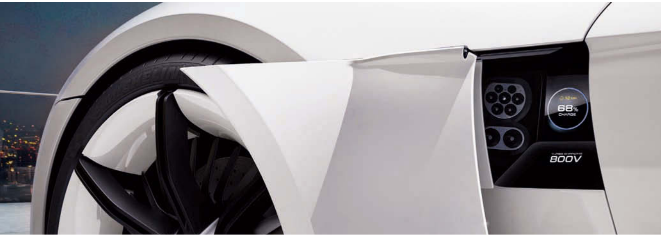
Moveable front wing reveals the 'Porsche Turbo Charging' port for fast charging of the Mission E
