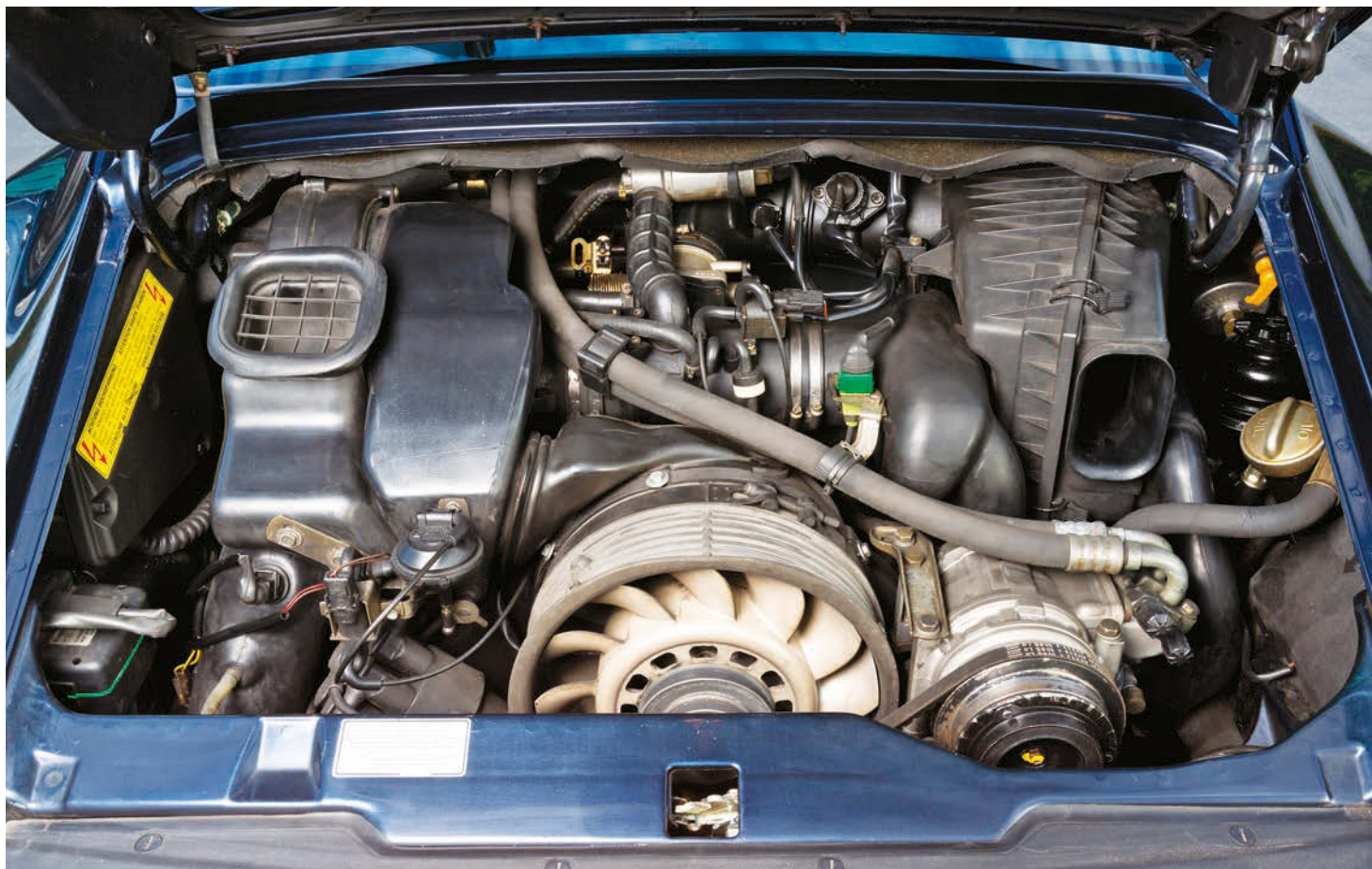
All 993 Carrera models were powered by a 3.6-litre flat-six motor – the last air-cooled Porsche engine. Later VarioRam engines produced 285hp compared to the earlier unit's 272hp
