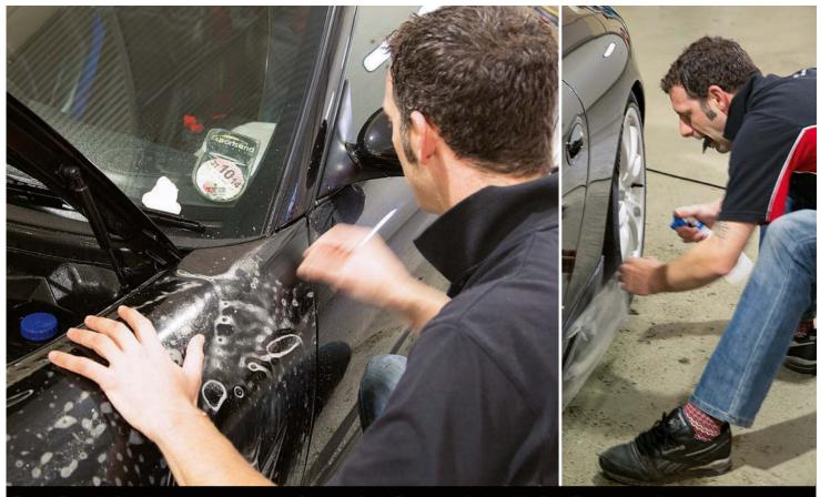
The latest film used by Paintshield has 100% clarity and with the fitters able to fold the film over a panel's edge it allows for the film to appear invisible once applied to the car's body
