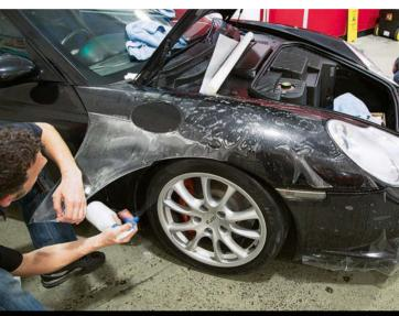
A slip solution allows the fitter to position the film precisely on the panel before it's fixed
