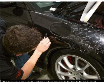
The fix solution reacts to the adhesive which then bonds the film to the body panel
