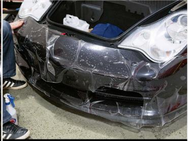
Excess solution is pushed out and a small amount of excess film is folded over the panel
