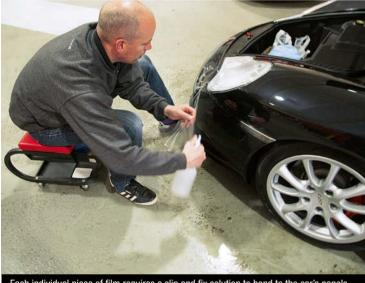
Each individual piece of film requires a slip and fix solution to bond to the car's panels
