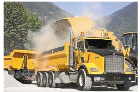
One of 16 550bhp T800 tri-drives used on the construction of facilities for the 2010 Winter Olympics staged in Canada.
