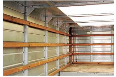
Close-up of the interior. The wood is for securing the payload and is not an integral part of the construction.
