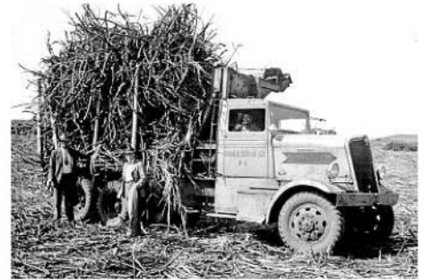
Following exports to Hawaii in 1936, sugar cane haulers became Kenworth's first 6x6s.
