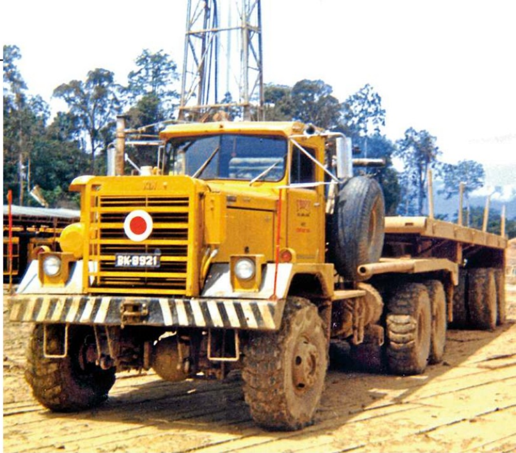
Built by Kenworth's former Canadian plant in Vancouver, top spec 849s could haul up to 250 tonnes.
