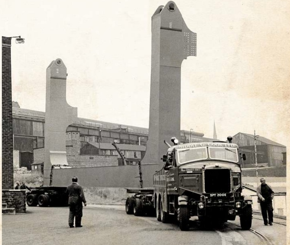
Arthur was requested to capture another internal move which dates from September 15, 1967. Siddie C Cook (which by then was part of the huge Road Services Forth organisation) used this virtually brand new Scammell Junior Constructor and a pair of steerable Crane Fruehauf bogies to make easy work of this awesome lump.
