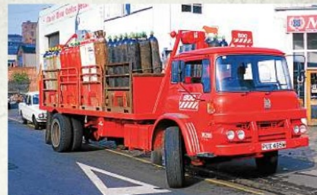
A more specialised load and corresponding bodywork is for the transport of compressed gas. The British Oxygen Corporation used a great many of these to carry oxygen and acetylene bottles etc, for use in industry. The fleet was always kept tidy and this example was pictured in the Sandpits area of Birmingham having come from Wolverhampton.
