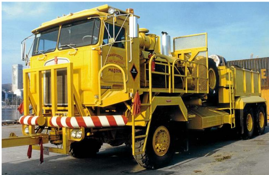
One of a trio of 993 6x6 extra-specials built in the early Eighties. The 700bhp Cummins is behind the cab. The operator was Spanish.
