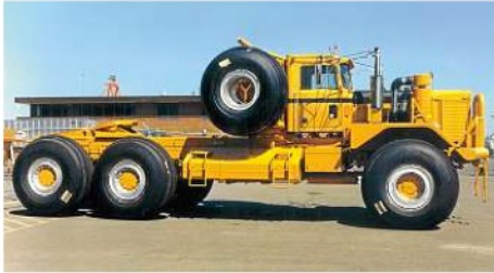
953 series oilfield trucks like this tractor unit were in production from 1958 until 2006. Tyres were up to 5.75ft in diameter.
