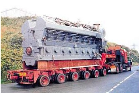
Renown at work. Note the trailer's axle configuration could be altered – there is no bed and the six axles are together PHOTO DAVE LEE.
