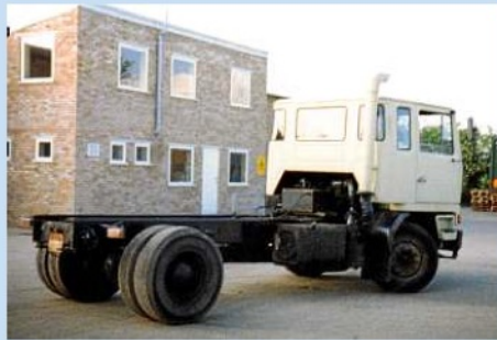
The TM had its chassis lengthened and a sleeper cab fitted before the TFL body and recovery gear was swapped over from the Bison.
