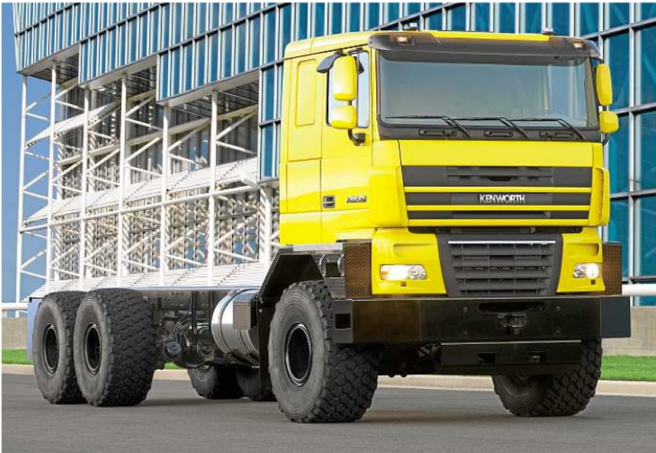
Cabovers being a thing of the past in the US, in recent years non-catalogued C500Ks have used DAF-sourced cabs.
