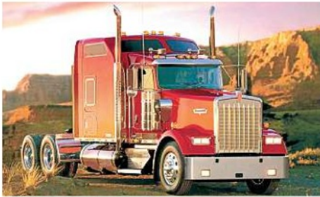
Subtle evolution: The classic lines of the current W900 depart from tradition with a single rather than two-piece windscreen.
