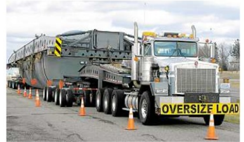
Spec'd for low-speed oversize load haulage, as the super-size radiator shell indicates, this C500 'tri' has extra cooling capacity.
