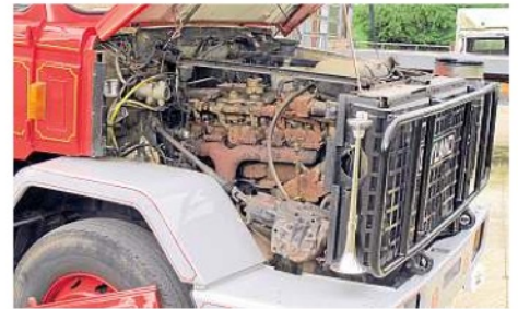
The 250 Cummins straight six was a customer option when the Landtrain was ordered new.
