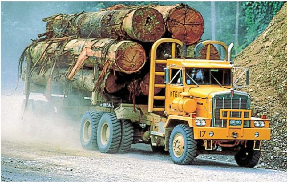
Kenworth logging-truck exports to Indonesia began in 1949. This 350bhp C520 is of late-Eighties vintage.
