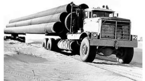
The legendary 853 desert oilfield 6x6 was initially designed for ARAMCO in the late 1940s.
