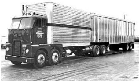
This early-Fifties 8x4 squeezed more payload volume within a regulation-limited overall length. The engine was midship, under the chassis.
