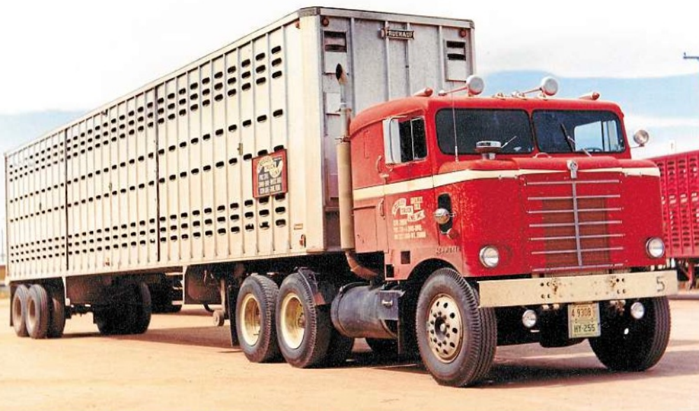
The 523 'bull-nose' cabover was introduced in 1949 and replaced by the K100 series in the early Sixties.
