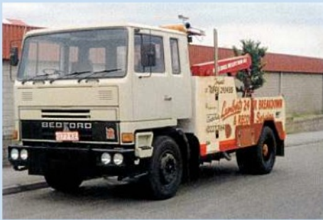
The TM had its chassis lengthened and a sleeper cab fitted before the TFL body and recovery gear was swapped over from the Bison.
