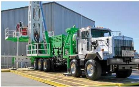
Typifying current heavy-duty production for the North American market is this twin-steer/tridem rear C500 oilfield rig.
