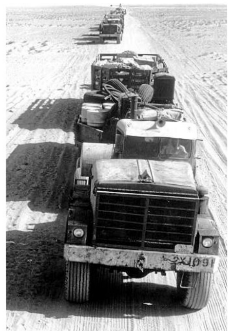
The original 853s featured 318bhp Hall Scott gasoline engines. Tyre specs were based on a camel's weight and hoof print area.
