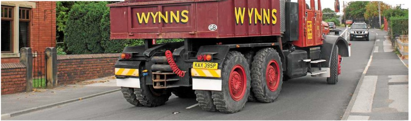
The temporary ballast box was made by Graham Booth, and is of the type used and made by Wynns to convert artic units into box tractors.
