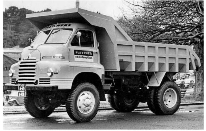
A short wheelbase R Type with dumper body used by Fletcher Construction.
