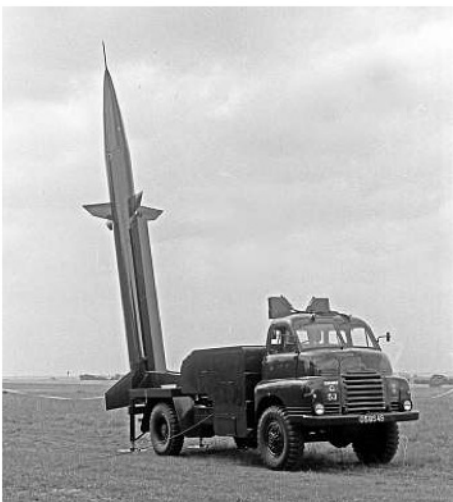
The British Army used the R Type in many different guises, including as a 'Blue Water' rocket launcher. PHOTO STILLTIME ARCHIVE.
