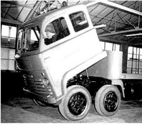
The X2 was ahead of the game in having a tilt cab – but with two engines to get at, it was a logical innovation.
