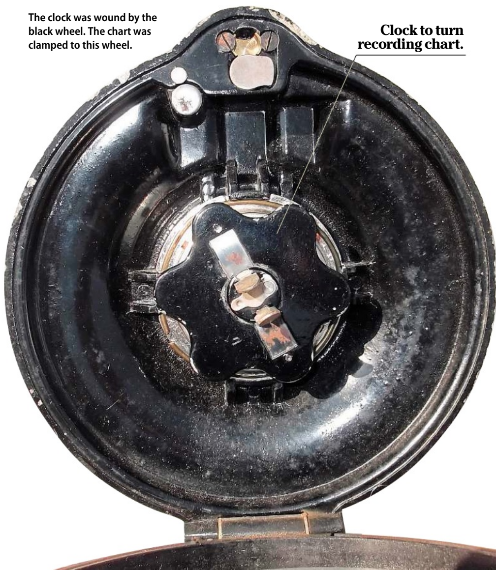
Not all Service Recorders had visible clocks, as some had a metal cover.
