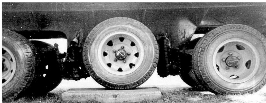
The chain linked suspension system with central spring pivoting caused upward forces to be distributed to the adjacent axle springs. This helped maintain constant road contact of all three bogie wheel sets.
