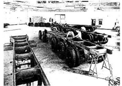
Four of the total of five X2 cabover-engine chassis built by Eisenhauser. Assembly took place in a building owned by a Louisville Chevrolet dealership.
