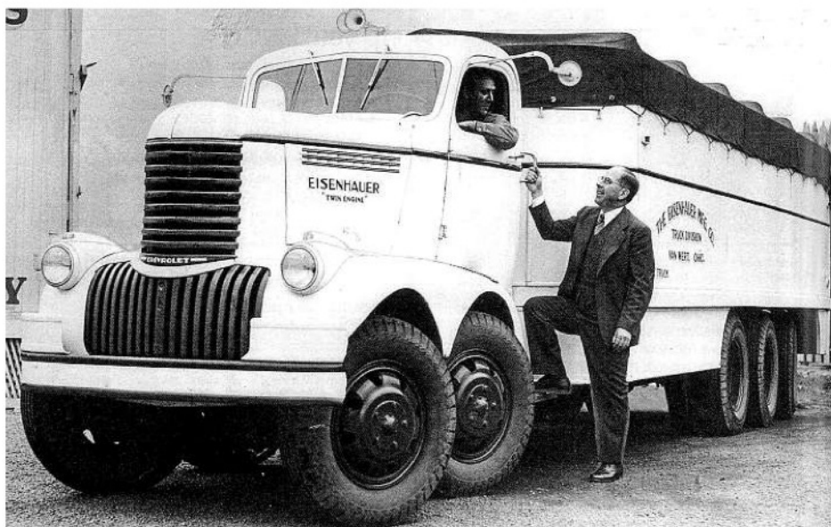
Photographed here in 1947, the Eisenhauer 10x4 Twin Engine Freighter had a designed payload capacity of 20 tons, higher than any other rigid truck of the period.
