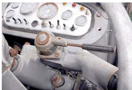
Air shift lever for the 3-speed auxiliary gearbox.
