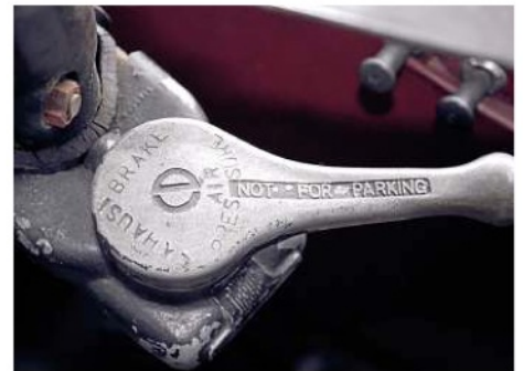
The Rolls-Royce engine has a butterfly flap-type exhaust brake activated by this hand valve on the side of the steering column.
