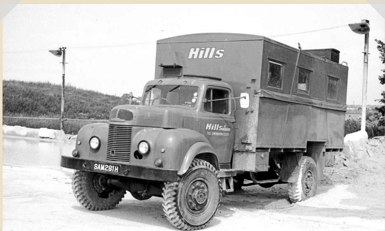
This ex-military Commer Superpoise 4x4 has found civilian work as a mobile workshop for Hills of Swindon, a company that is still very much with us specialising in quarrying and waste management. NA3T photo CX00366.
