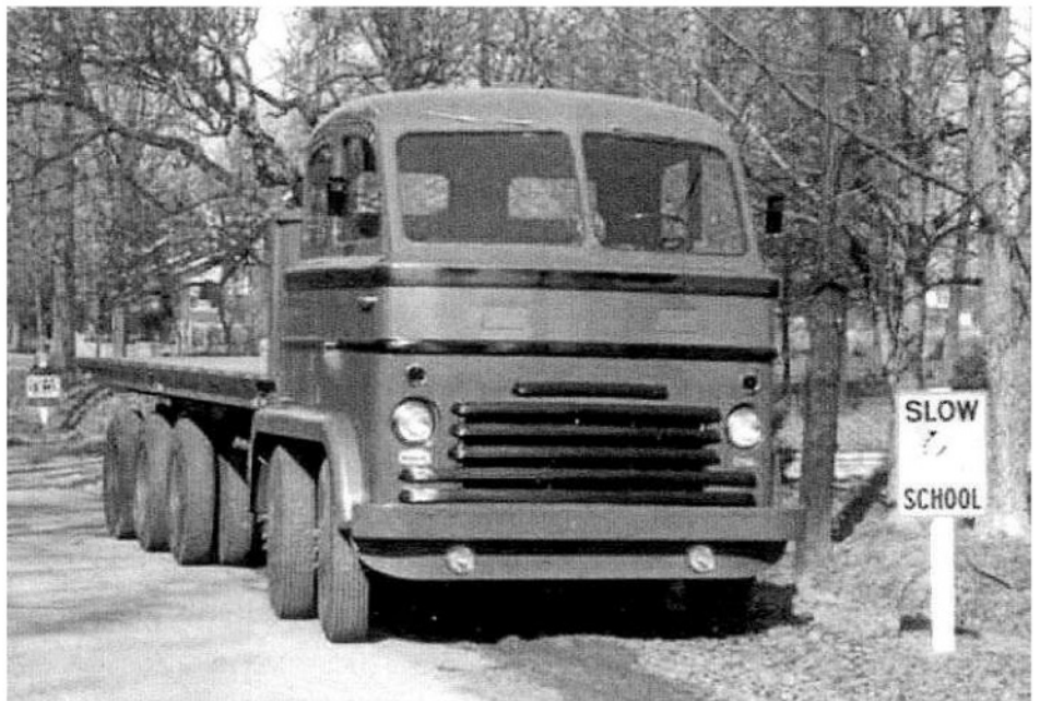
The X2 was engineered to overcome inefficient truck and trailer designs dictated by state highway vehicle regulations. A study by Eisenhauser concluded that ill-thought out laws made an unintended contribution to highway and bridge deterioration.
