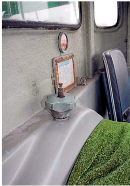
This screw down lock stops the cab tilting.
