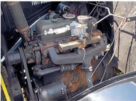
The LC3 is powered by a 2050cc ohv four-cylinder petrol engine developing around 42bhp.
