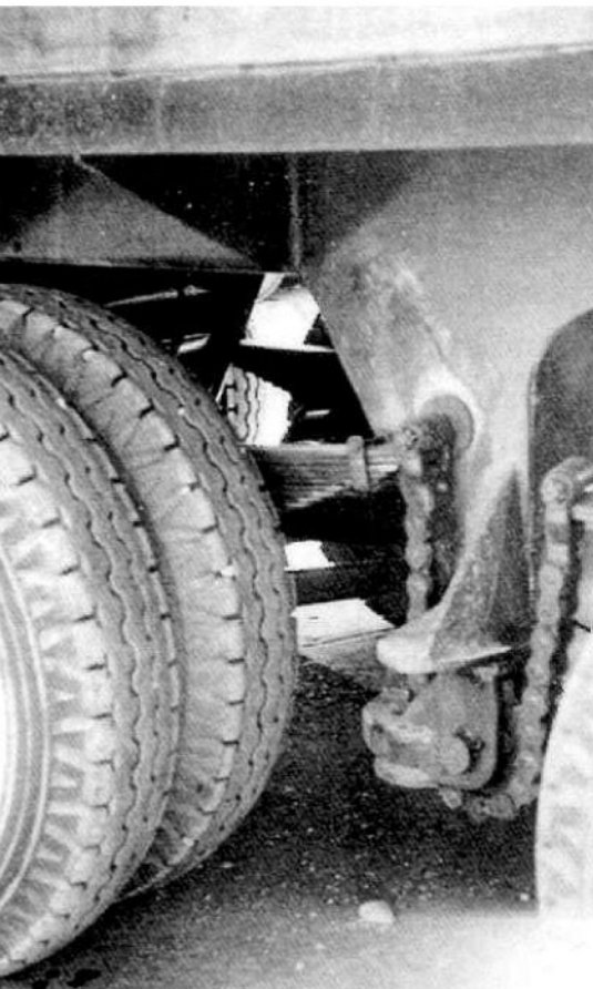
The rear axle articulation setup incorporated a flexible chain arrangement connecting the tandem leaf spring and the leading suspension arm, which pivoted on a ball-joint.
