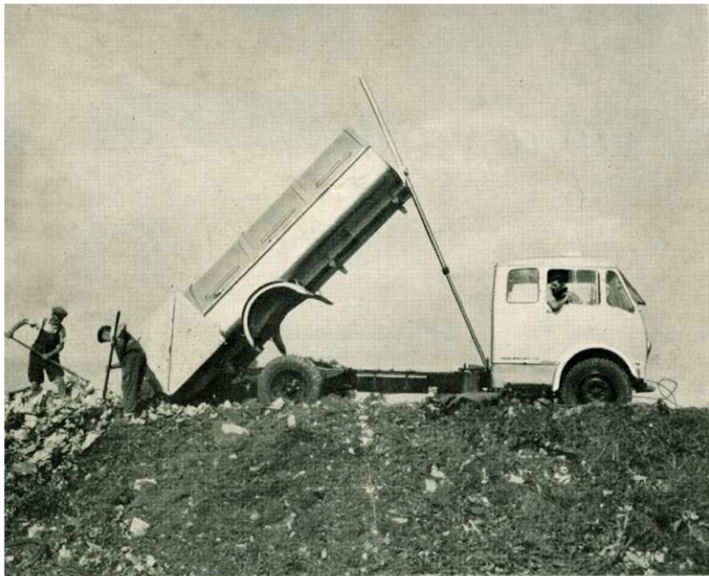
Tipping gear on the 10 cu. yd. model is operated from the cab. A tipping angle of approx. 45° ensures ease of unloading.
