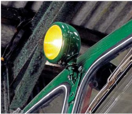
This small yellow beacon was activated when the ERF was on the road to mark its slow progress.
