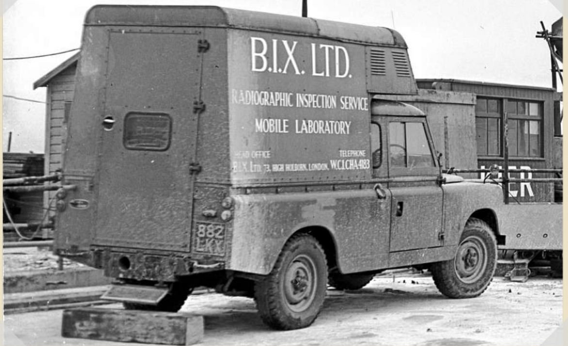
This Series 2 long wheelbase Land Rover was used as a mobile laboratory, and was photographed in the mid 1960s on the construction of the M2 in Kent. BIX Ltd did radiographic testing to discover flaws, cracks etc in welds and materials. NA3T photo GM00328-Bd1.
