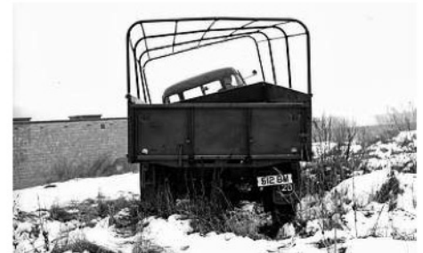
RL under test. Note frame/body flex.
