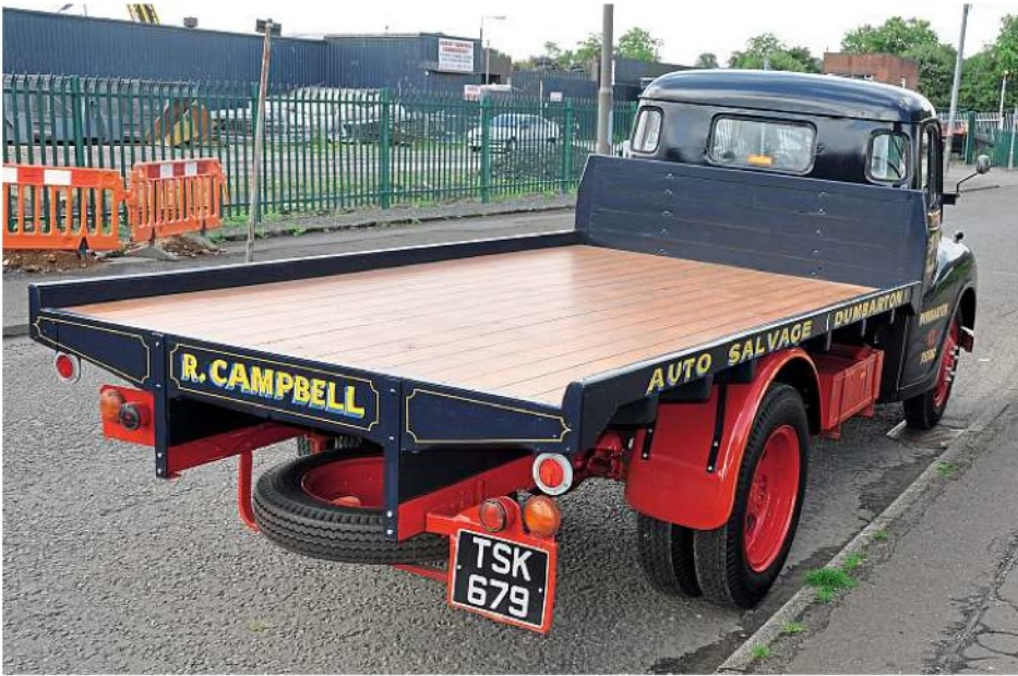
The wooden flatbed had to be re-created using the Austin's original metalwork.
