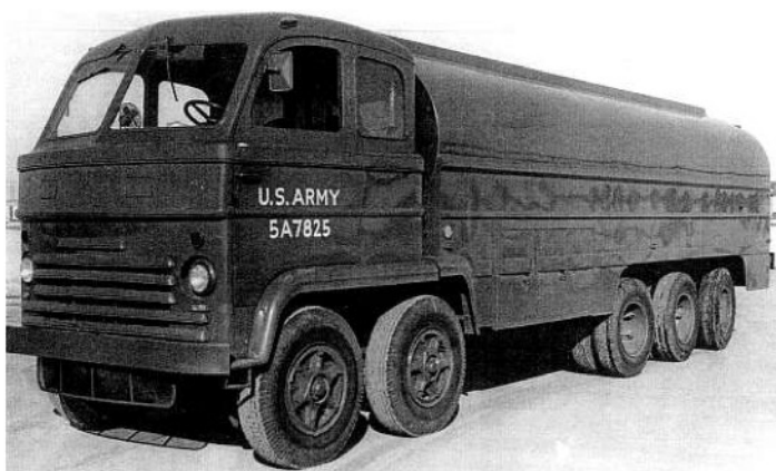
Fitted with a 6176 US gallon tanker body, an X2 was purchased for $20,000 by the US Army in 1956 and successfully tested at Aberdeen Proving Ground in 1957.
