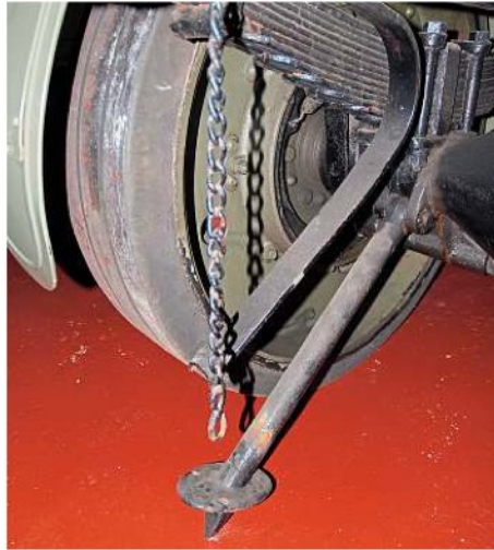
The ‘spragg brake’ to prevent the vehicle running away backwards.
