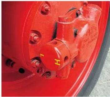
The change mechanism for the high and low hubs Foden used to fit on the heavy haulers.
