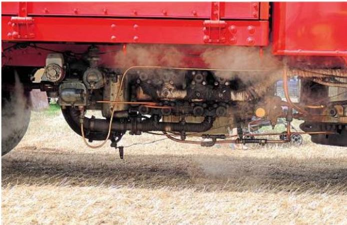
The undertype steam engine installation allowed a longer loadbed within a given overall length.
