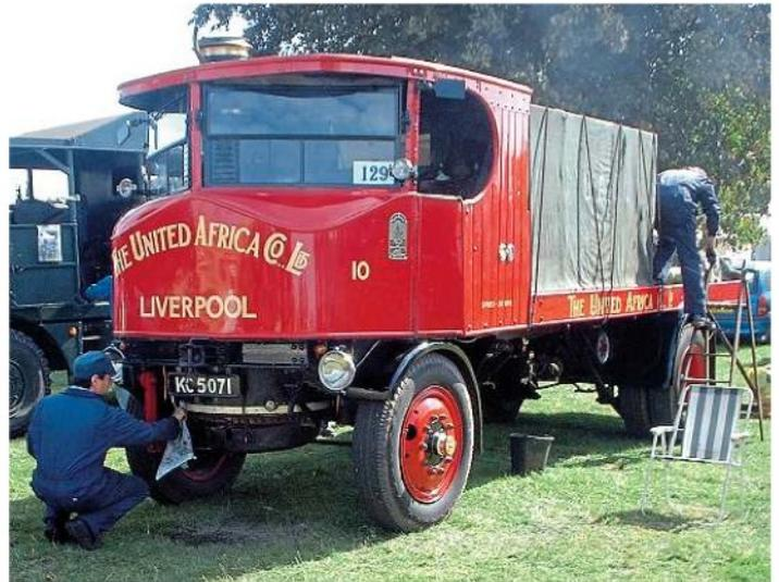
A restored 1924 'Super' platform truck; pneumatics were the norm from the beginning of the 1930s. Older vehicles were upgraded.
