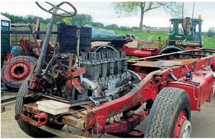
Cab off, and work starts on the chassis and engine. PHOTO JOHN AND NEIL BOUGHEY.
