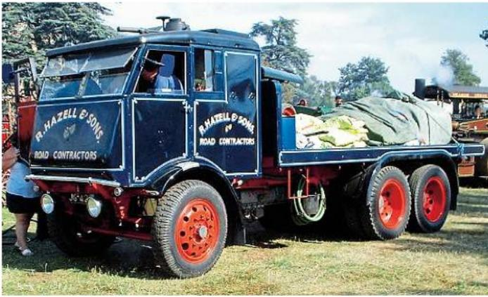
With the all-important get-it-where-you-can water tank hose clearly visible, a pristine S6, the most advanced steam truck design ever put into quantity production.
