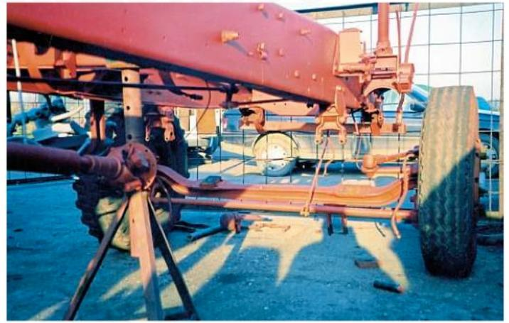
The chassis cleaned, repaired and painted, and the front axle can be refitted. PHOTO JOHN AND NEIL BOUGHEY.
