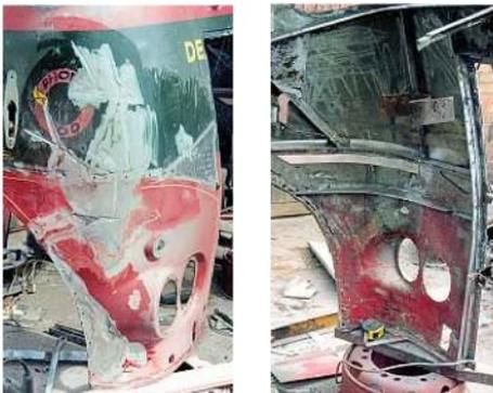
Repairing the Boalloy cab. Some of the internal framing had to be replaced, together with a completely new rear panel. PHOTOS JOHN AND NEIL BOUGHEY.
