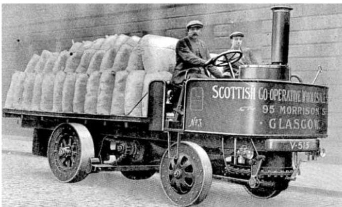
A 'Standard' type, delivered in 1907: in 100,000 miles, this particular wagon reputedly required only one day off for maintenance.
