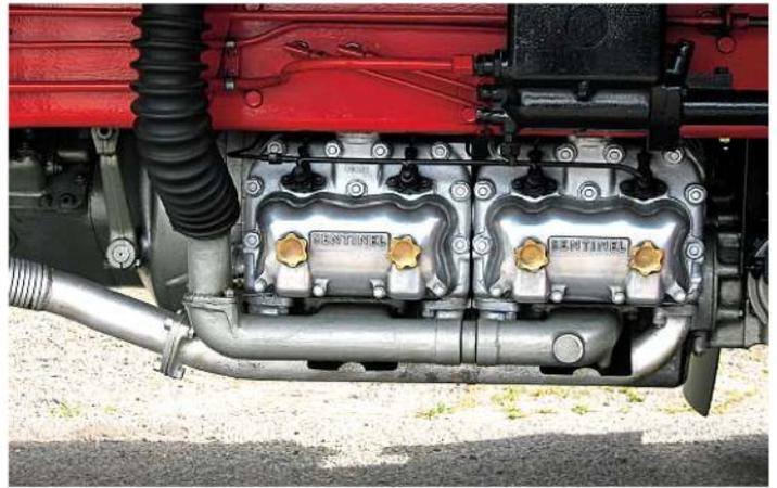
Sentinel's under-chassis mounted horizontal 4-cylinder, 6.08 litre diesel developed maximum power and torque outputs of 82bhp and 259lb-ft.
