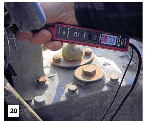
20 I then checked the live feed to the switch and this showed green indicating that it was live. I then checked both dip and main beam wires and these proved okay.
