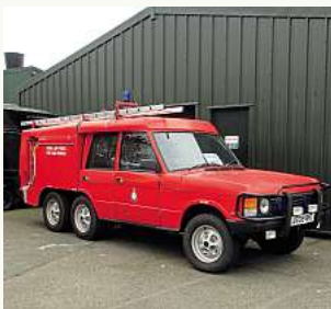
This ex-RAF six-wheeled Range Rover provides the fire cover when taxiing the Lancaster 'Just Jane'. PHOTO SUE CREASEY.
