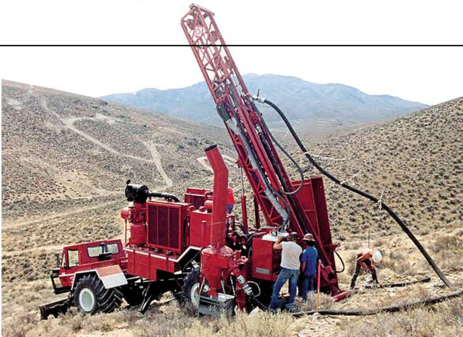
Designed for drilling on steeply sloped terrain, the Explorer 1500 drilling rig carrier incorporates hydraulic deck levelling and a dozer blade ground anchor.
