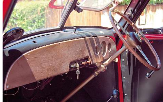
The GPO early wooden dash was also an option for 'civilian' LCVs.
