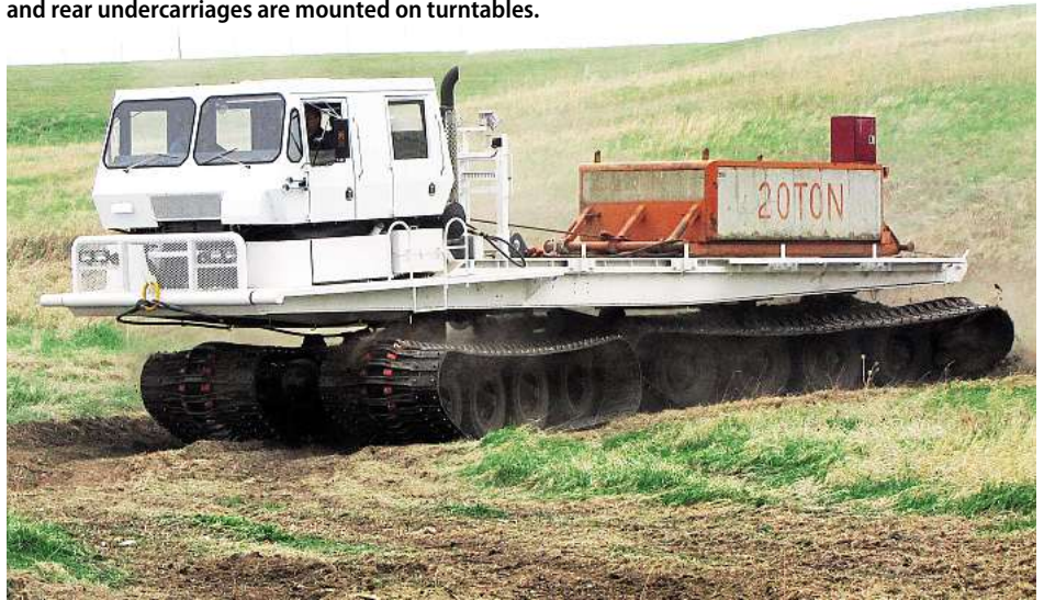
Under test, a Husky 8 rigid with the current cab. The front and rear undercarriages are mounted on turntables.
