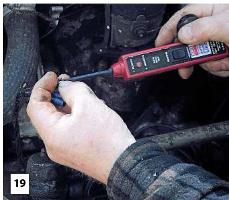
19 Tracing a fault in a headlight circuit, I first tested the earth wire; here the LED showed red (positive). This vehicle is positive earth so it's correct.
