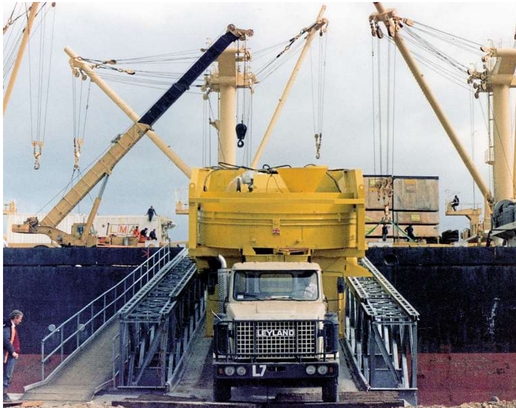
Leyland number L7 brings a load down the section of Bailey Bridge from the Merchant Providence jetty.
