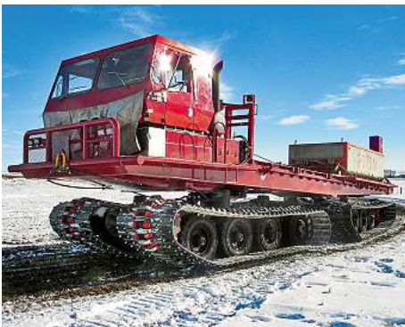
A truck on tracks: current spec Husky 8 4-track transporters have a 440bhp CAT diesel. Designed gross is 87.25 tons.
