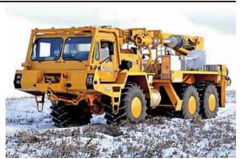
A pivot-steer 6x6 Delta 3 with extra cab protection structure. Fitted with a digging derrick, it was supplied to Manitoba Hydro in 2010.
