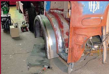
January 2014, and the cab resto begins in earnest. At the primer stage.
