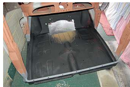
An LCV with the cab removed – note the flat floor.
