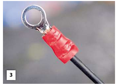
A crimp-on terminal, as intended, crimped on to the wire end. Functional but not very pretty.
