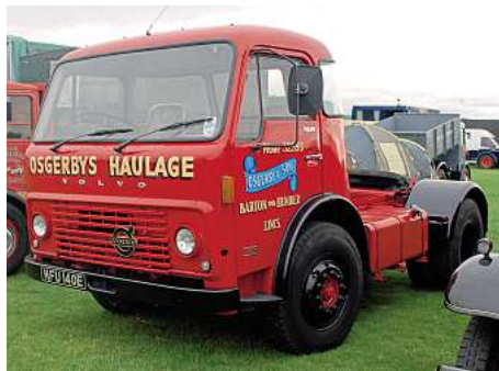
Having been registered on June 13, 1967, this F86 tractor unit was one of the first Volvo lorries ever to be officially sold in the UK. It was supplied complete with a 33ft York trailer by dealer John Hebb of Wootton, and was used at 32 tons mainly on fertiliser deliveries.
