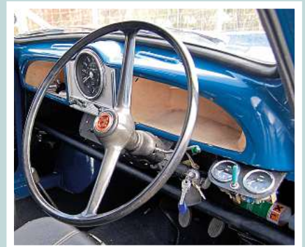
The Series V dash for LCVs – note the lack of glove box lids.
