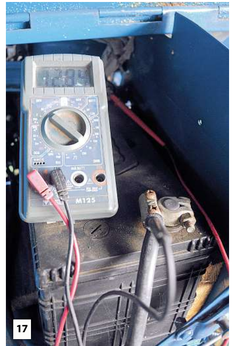
17 This tractor is showing a much healthier 12.84v after standing for about a month. I'm sure this is a good battery and the tractor will fire up.
