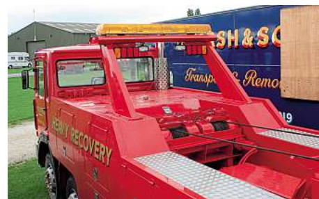
A large hydraulic tank is concealed in the bodywork behind the cab to operate any stricken tipper mechanism.
