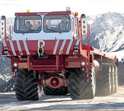
High, wide and handsome at 14ft 7in tall and 12ft wide, the 8x8 Commander Tri-Axle has a designed gross of 84 tons, at which weight ground over-pressure is only 14.4psi at 3in surface penetration.
