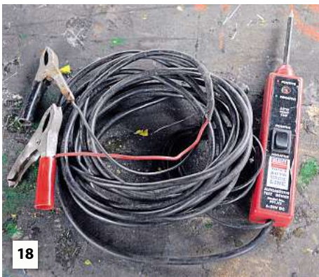
18 This is a power probe used in the motor trade, and it has several useful features. It is clipped onto the vehicle battery, the probe can then be placed on a suspect circuit connection and the LED will illuminate either red or green depending on the voltage potential.
