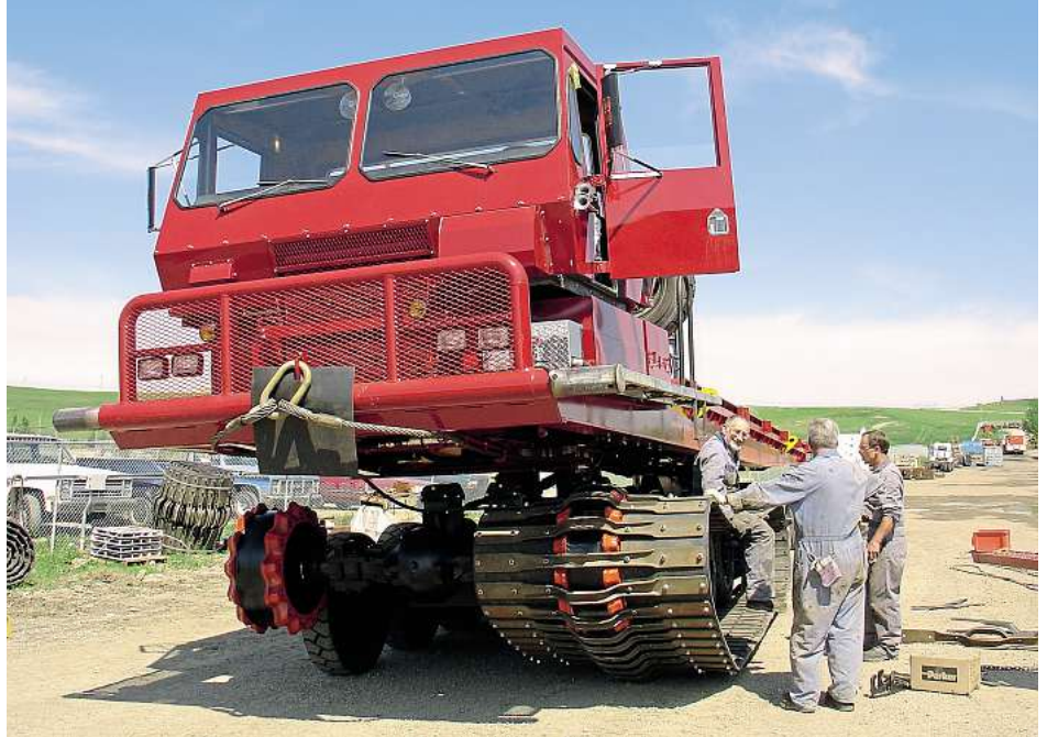
The ground pressure imposed by a man standing is upwards of 8psi. At full load with 6in surface penetration, ground loading of the Husky 8 is only 4.62psi.
