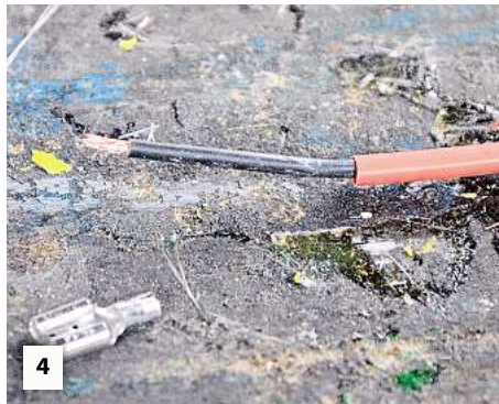
My preferred way to make the connection is to solder the crimped terminal minus the insulation; this gives the best of both worlds, a mechanical connection (crimp) and a soldered connection keeping out moisture.
