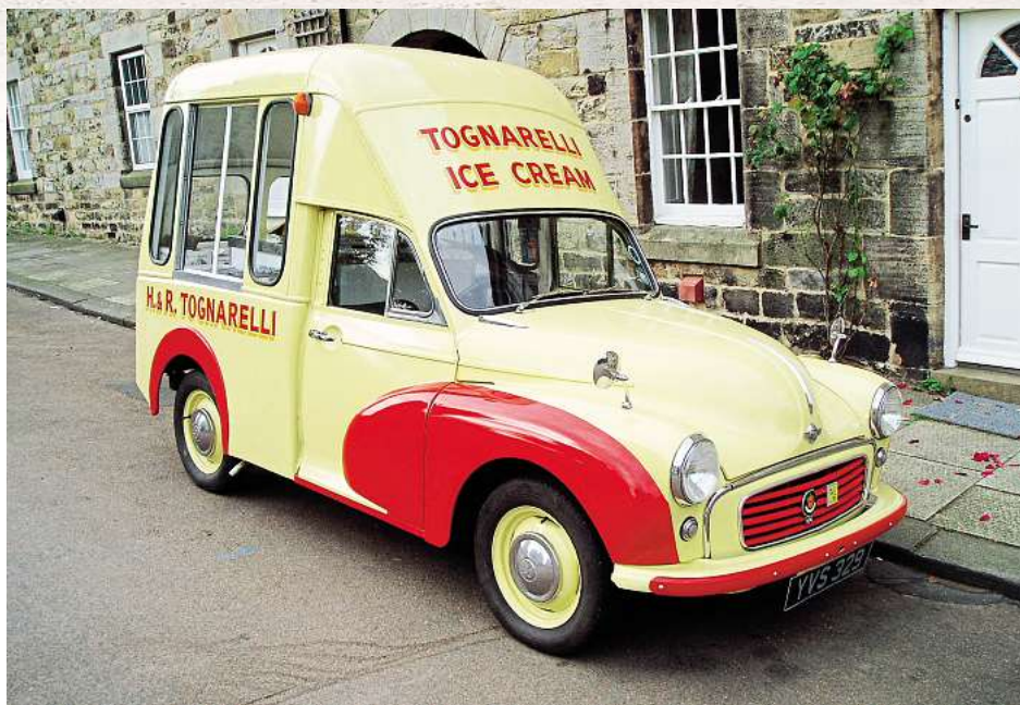
The separated chassis allowed special versions to be constructed by outside coachbuilders.
