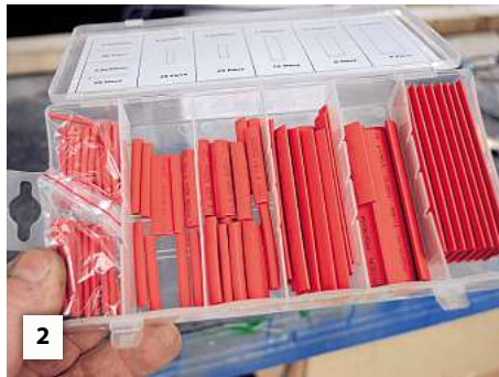
Heat shrink sleeving is indispensable for making a good dry insulated connection.
