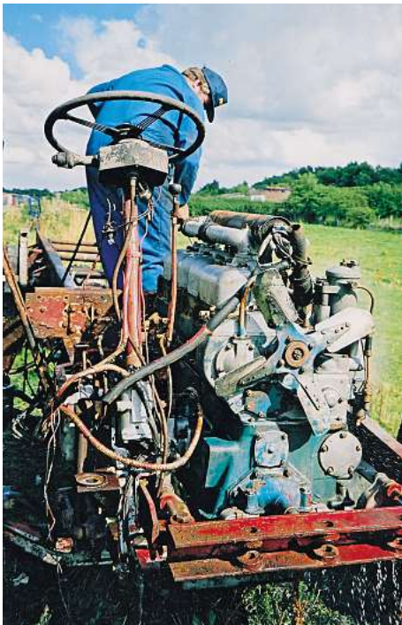
David steam cleaning the engine during the strip down. PHOTO DAVID PHILP COLLECTION.
