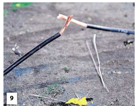
A straight splice is often needed in a loom to extend a broken wire etc. Strip the insulation back on both wires, make sure that bright copper is showing otherwise solder will not adhere.
