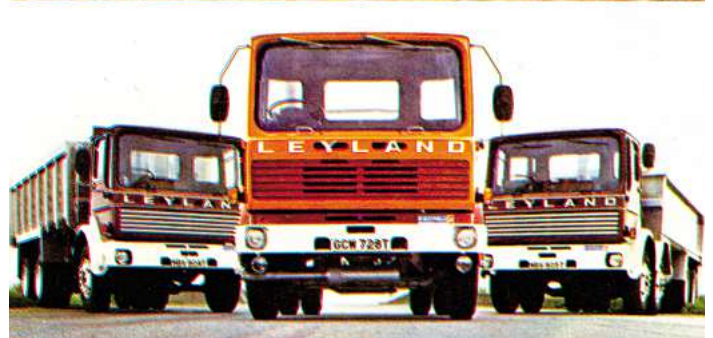
Reiver 24 ton GVW – biggest selling 6 wheel tipper – high payload – it carries 3 times its own weight with double drive rear hub reduction axles for on/off road use.
