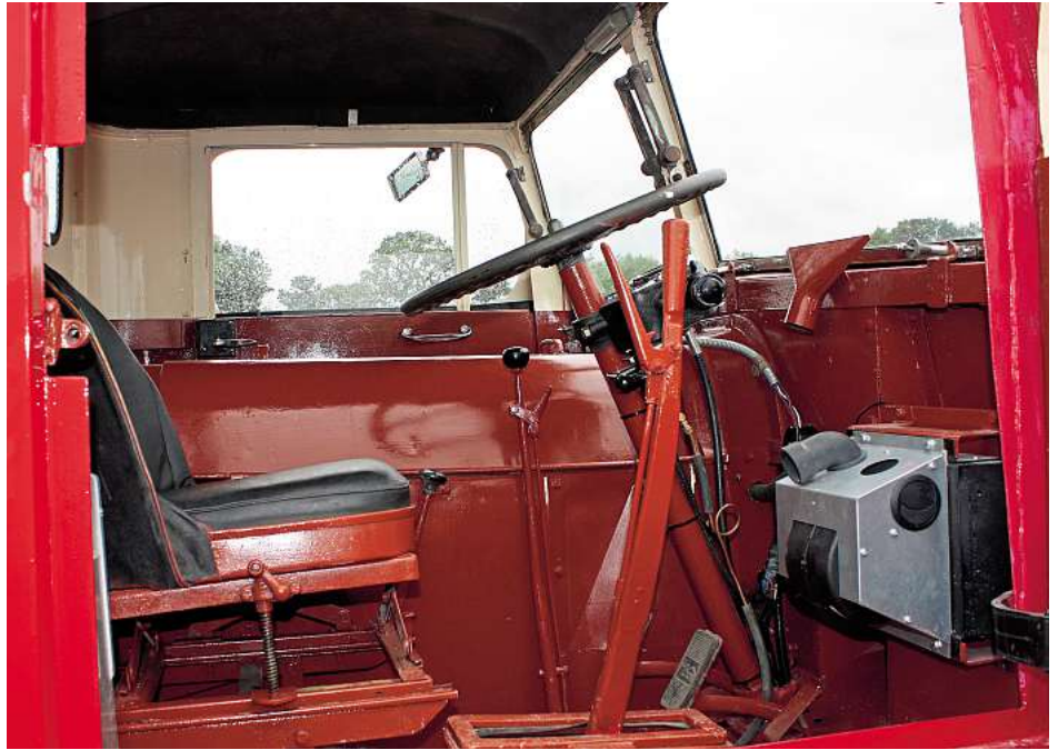
The interior is certainly not weighed down with too much trim. The heater has yet to be finished off and piped in, and the small gear lever down by the engine hump – to the left of the driver – is for the extra booster box.
