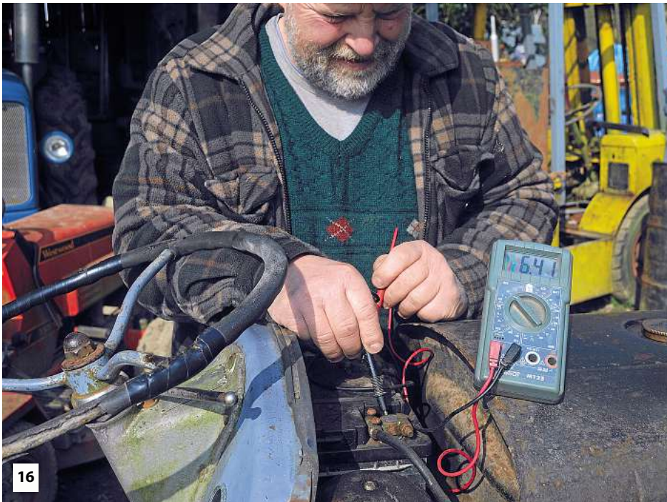
16 I thought I would check out the battery on this tractor as last time I started it, it was very sluggish. Not surprising with this reading, it looks as though a new battery is in order; however I will give it a long trickle charge and retest it before replacing.
