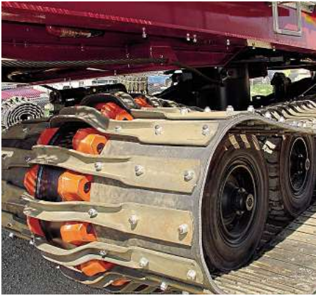
Foremost grouser-type tracks run on rubber tyred idler wheels. Combined with high track flexibility, the system ensures compliant ground contact for balanced over-pressure.
