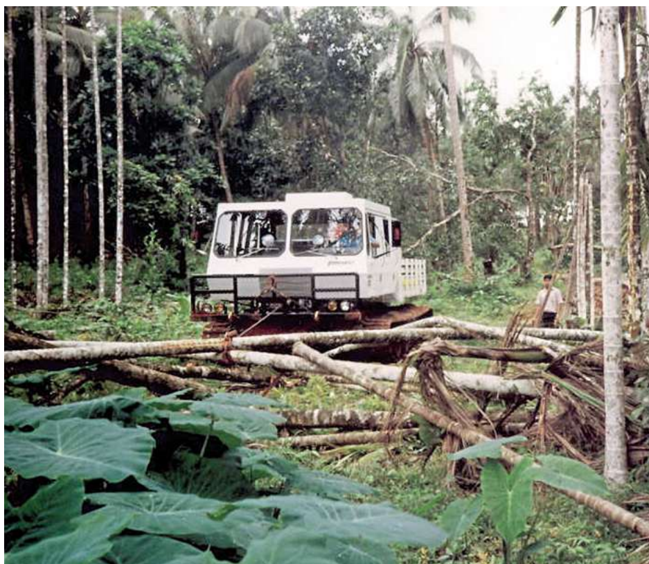
A Nodwell 110 of the current generation operating in the Burmese jungle. The payload is now 11.5 tons, more than double the original spec.
