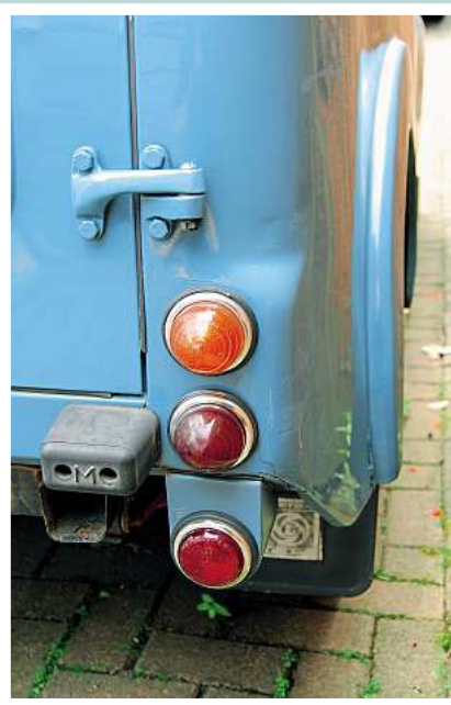
The panels around the rear light clusters suffer due to water being sprayed up from the wheels. It has to be cut out and a repair panel welded in.
