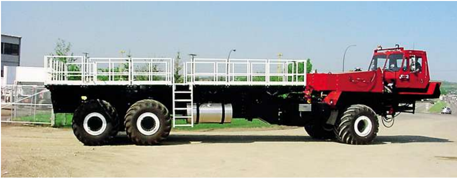
The biggest truck in Antarctica? This Commander C has a back-to-front reversed cab, customised for launching sub-orbital scientific balloons.
