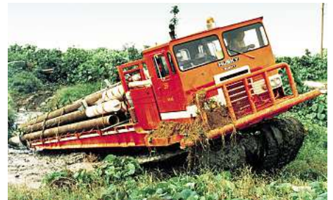
The first Husky 8 model was produced in the late 1960s. This example has the original in-house designed and built cab.
