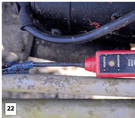
22 At the other end of the wire it showed green (negative) correctly, the switch on the power probe can be used to supply a positive or negative current so that suspect items can be powered up independently. It has an overload trip in the unit so that no harm will be done if a short circuit occurs.
