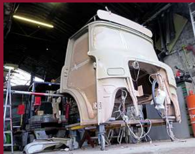
January 2014, and the cab resto begins in earnest. At the primer stage.
