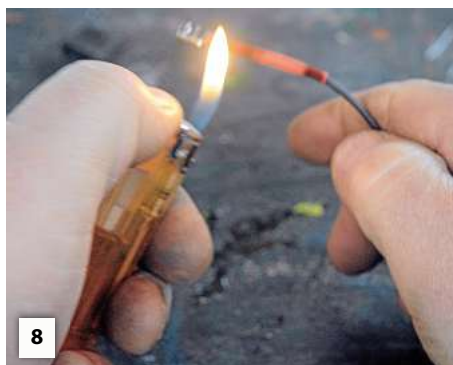
Use a heat source to shrink the sleeving tight onto connection; a lighter is ideal, although be careful if working near the fuel tank, in this case heat from the side of the soldering iron will work.
