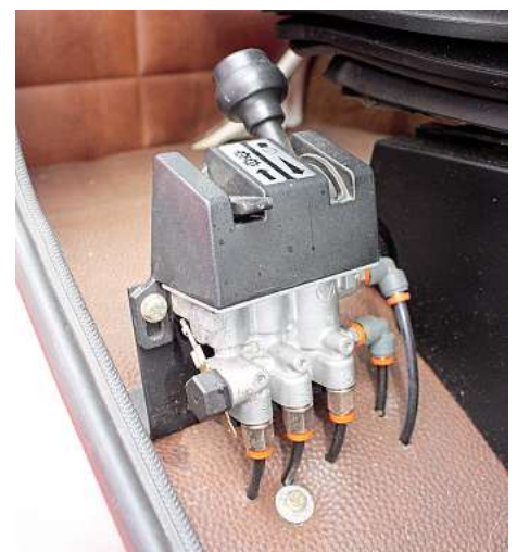
This PTO switch operates the tipper mechanism of a stricken vehicle if the hose is connected up.
