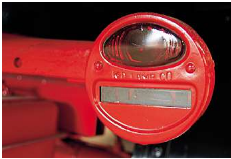
The rear lights are throwaway units made by the KD Lamp Company of Cincinnati, Ohio, USA.
