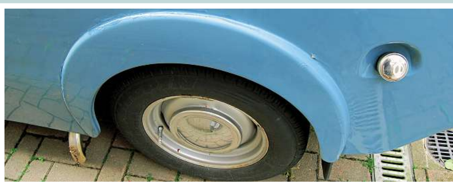
Wheel arches are a common rot spot and the arch has to be cut out and a replacement inserted.
