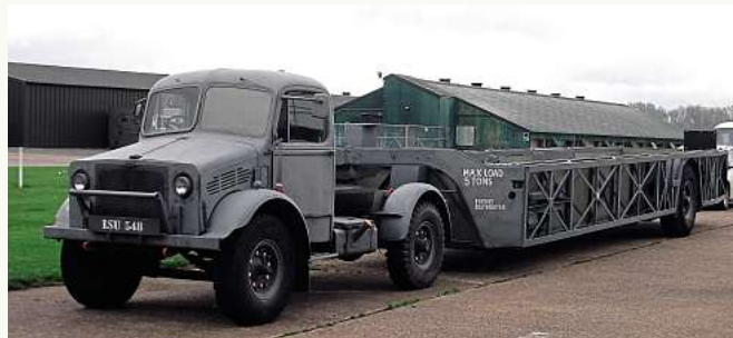
The Bedford 'Queen Mary' was used to move large aircraft sections. PHOTO SUE CREASEY.
