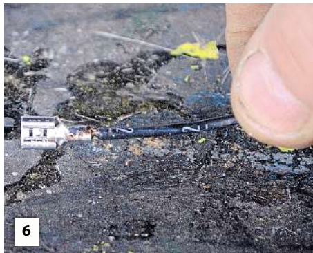
Soldered and crimped terminal ready for the heat shrink sleeving. Wait until cooled before sliding it over the joint, otherwise the sleeving may shrink before in correct position; remember to put the sleeving on the wire before fitting terminal.
