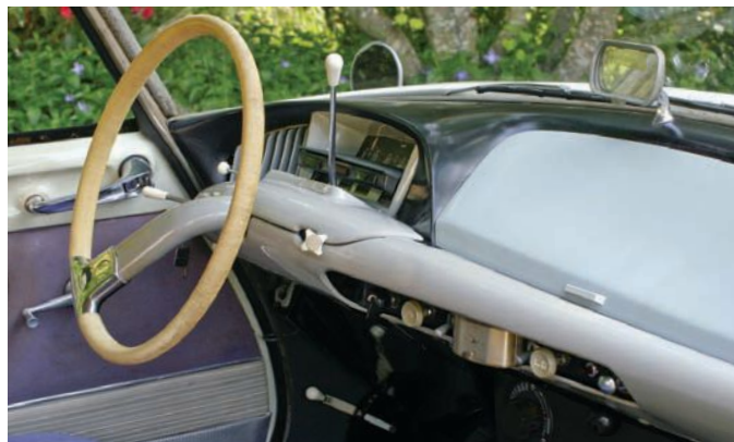
Bertoni's radical original dashboard was then the largest single-piece nylon molding in the world, and the one-spoke steering wheel was a safety feature that became a Citroën hallmark.
