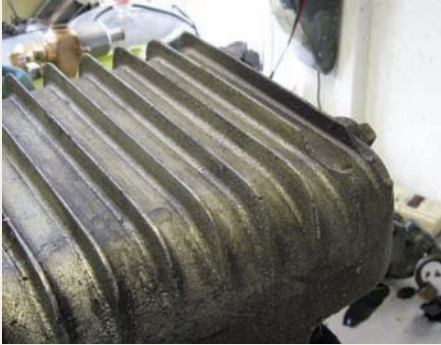
8 The MG's engine features a squat, finned aluminum sump that can hold five quarts of oil. Broken fins were repaired with TIG welding, but no serious cracks were found.
