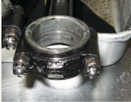
9 Engine disassembly allowed the shop crew to look for manufacturing marks on components, including connecting rods. This was done to verify that the internals were factory-original from correct supplier.
