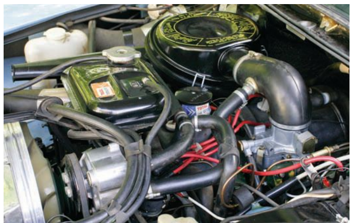
The DS 21's 2,175-cc, 115-hp four-cylinder would be the most powerful fitted to a U.S.-spec DS before imports stopped in 1972; later models could have 2,347-cc and 141 fuel-injected hp.
