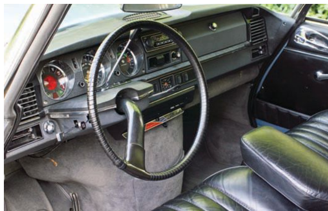
A more conventional instrument panel arrived for 1970, bringing easy-to-read round gauges, including a tachometer. Leather upholstered the "Dunlopillow" foam-cushioned Pallas seats.
