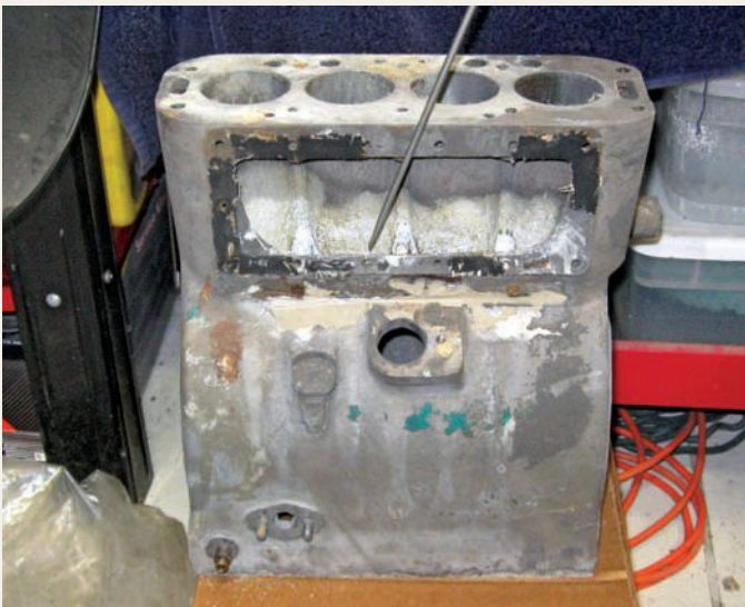
10 The block was found to have cracked around the bottom of the cylinder bores, where it's weakest, and was welded. The bores were badly damaged by corrosion and the electrolytic reaction with the alloy pistons, and had to be sleeved.
