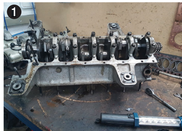
ABOVE The Ferrari 250 GT Boano like many racing engines has a 'dry' sump resulting in a lower centre of gravity and therefore better handling. The smaller sump also contributes to a lighter engine. This is the engine at the very first stages of strip and assessment
