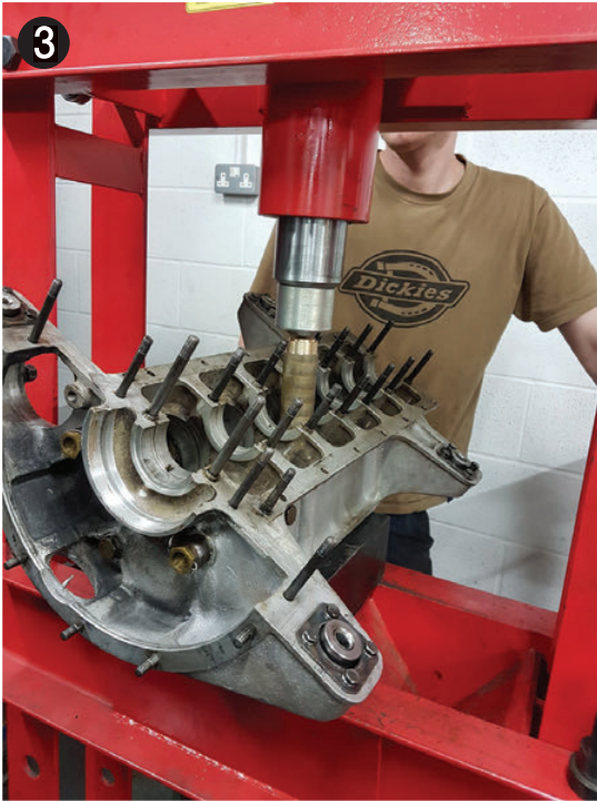
ABOVE Removing the liners. These were found to be in need of re-boring, a regular in-house service
