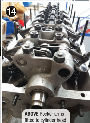
ABOVE Rocker arm reassembled
