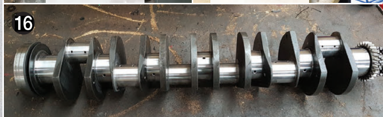
ABOVE 'Nitrided' crank re-ground. Formhalls noted this particular crank had been ground before, resulting in poor radiuses and big-end pins at different over-sizes to one another. It has now ground this crank and all journals are within 0.0005" tolerance across the whole shaft.
