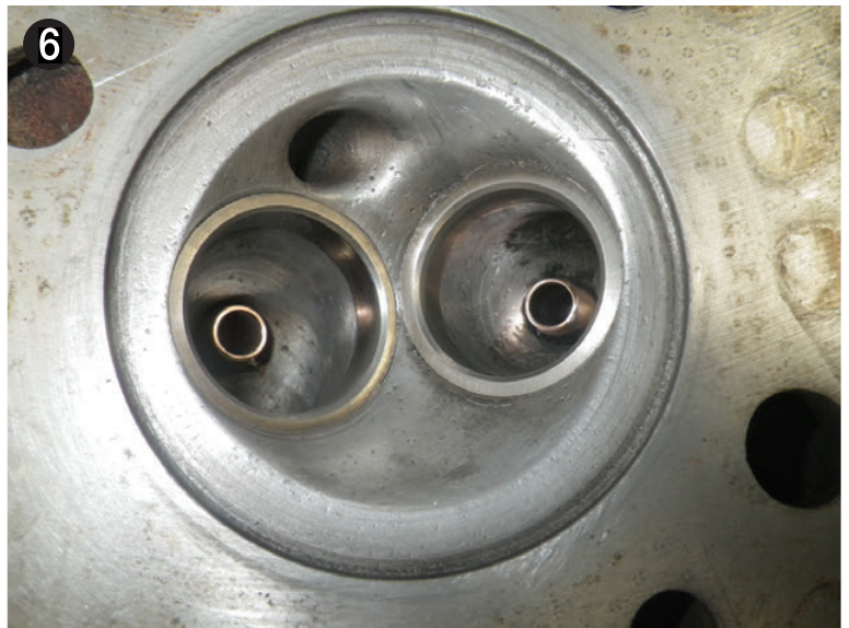
LEFT & ABOVE Valve seats before and after decoking and cutting. Formhalls offers a very wide range of in-house traditional manual machining. Cutting valve seats is standard procedure in its shop. The valves of this particular engine are cut to 45 degrees
