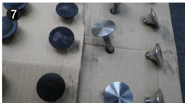
LEFT & ABOVE Valve seats before and after decoking and cutting. Formhalls offers a very wide range of in-house traditional manual machining. Cutting valve seats is standard procedure in its shop. The valves of this particular engine are cut to 45 degrees
