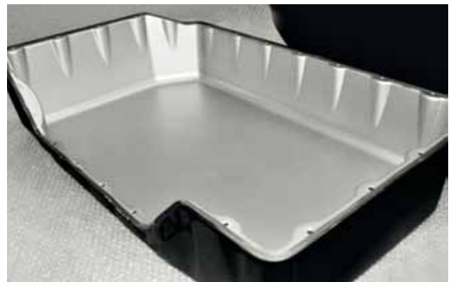
The cover of the battery is specially coated in order to protect it from electromagnetic waves
