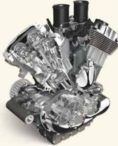
On the road since 2002: the 115 hp V2 engine for the "V-Rod" by Harley-Davidson
