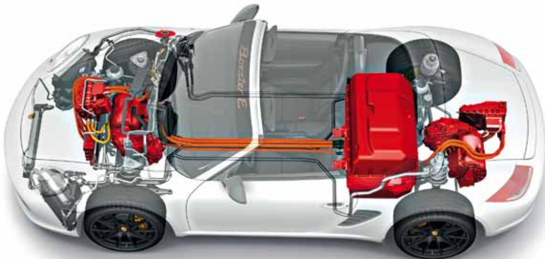
In the version with two electric machines, the Boxster E research vehicle reaches an effective output of 180 kW
