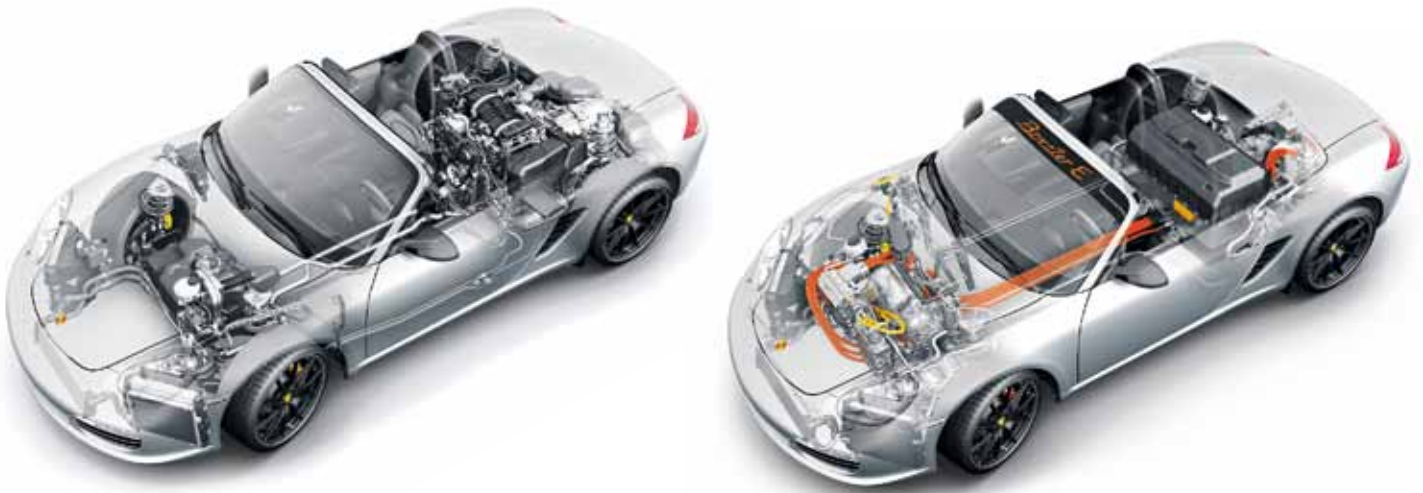
The battery in the Boxster E research vehicle is positioned in the same position as the mid-engine of the series vehicle
