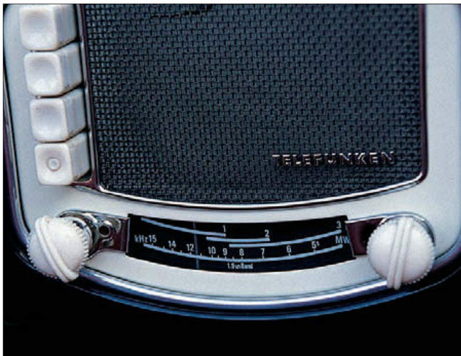
One of the options for the new 1952 cabriolet was a Telefunken push-button radio with built-in speaker. Although it took some time for the tube-type radio to warm up, it had good reception. The antenna was hidden inside the driver's side-view mirror.
