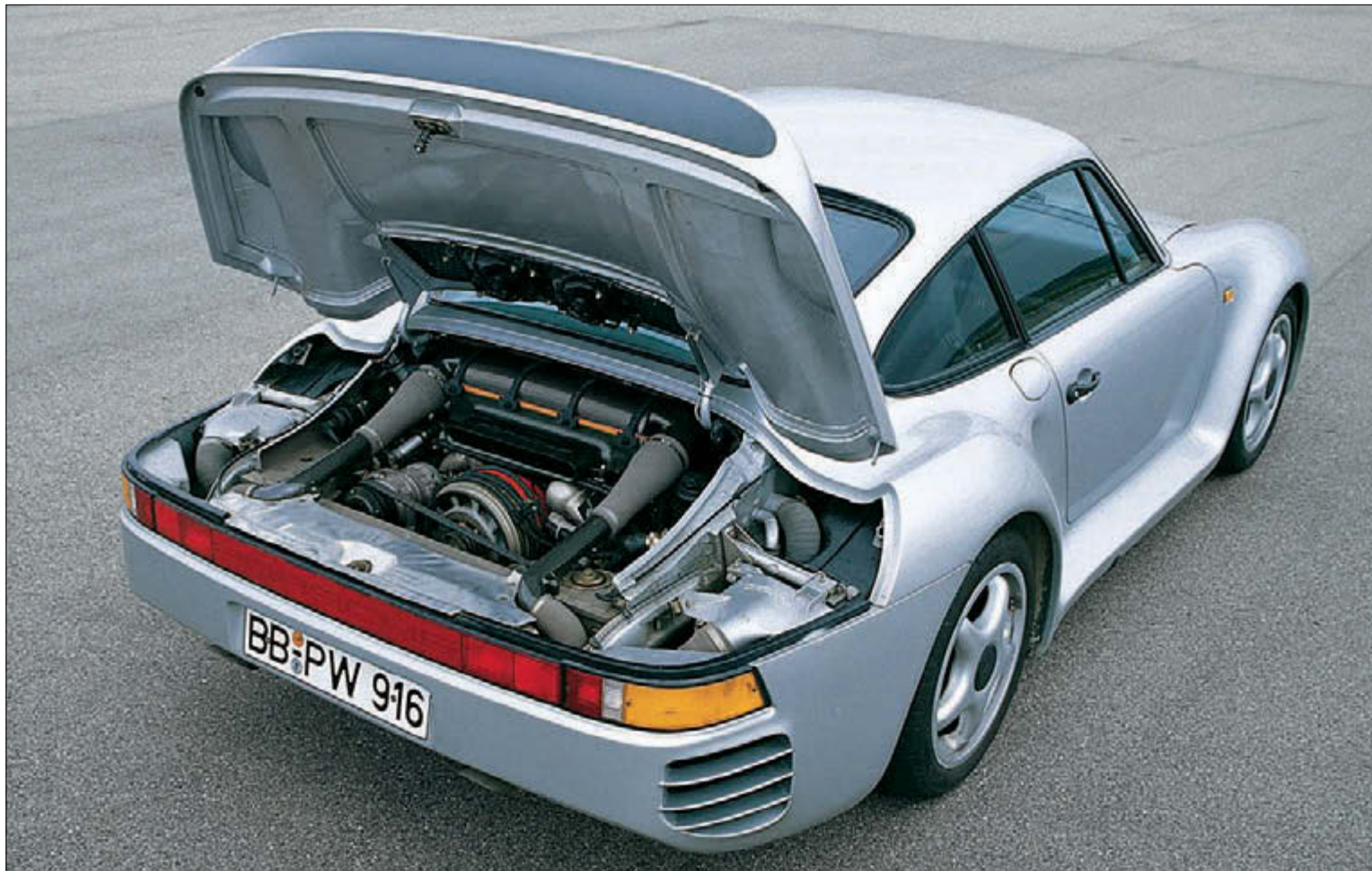
Under the rear wing and deck lid was Porsche's most sophisticated air-cooled engine. The limited production 959s produced 450 brake horsepower. (PORSCHE WERKFOTO)
