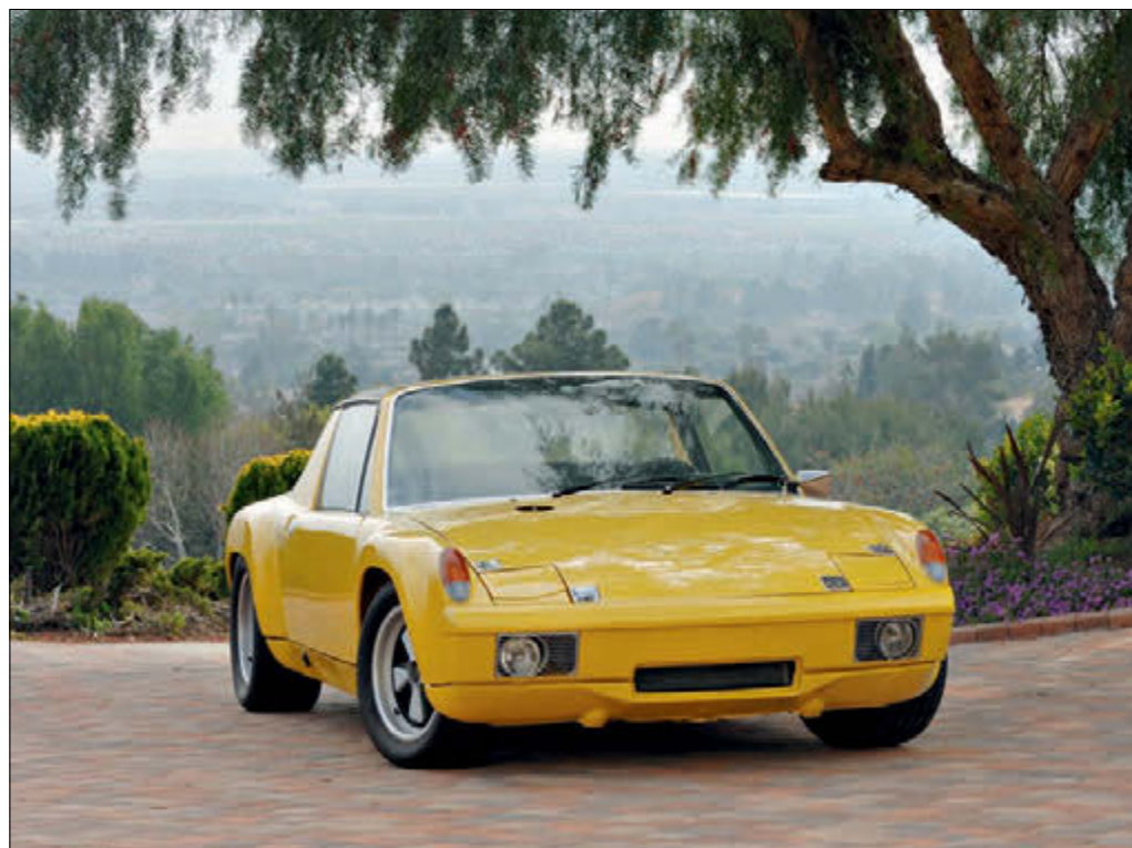
In the U.S., Porsche + Audi referred to these as 914/6R models. Each came with the "R Competition Option Group." With widened steel fenders to accommodate 15x7 wheels in front and 15x8 Fuchs alloy wheels in back, oil cooling, 100-liter fuel tank, racing seats, "specific suspension," a "changeable gear transmission," performance exhaust, and the 911S braking system, Porsche charged $15,568 for this car. (RANDY LEFFINGWELL)
