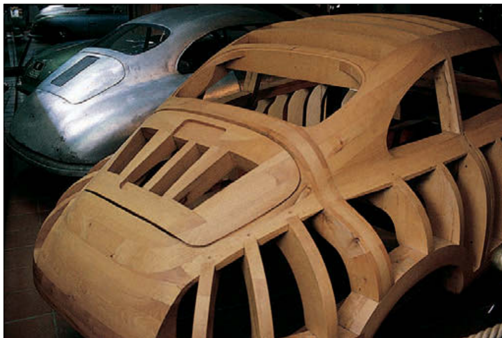
The original wooden styling buck for the 356-2 body is now displayed at the Porsche museum in Gmünd. (PORSCHE WERKFOTO)
