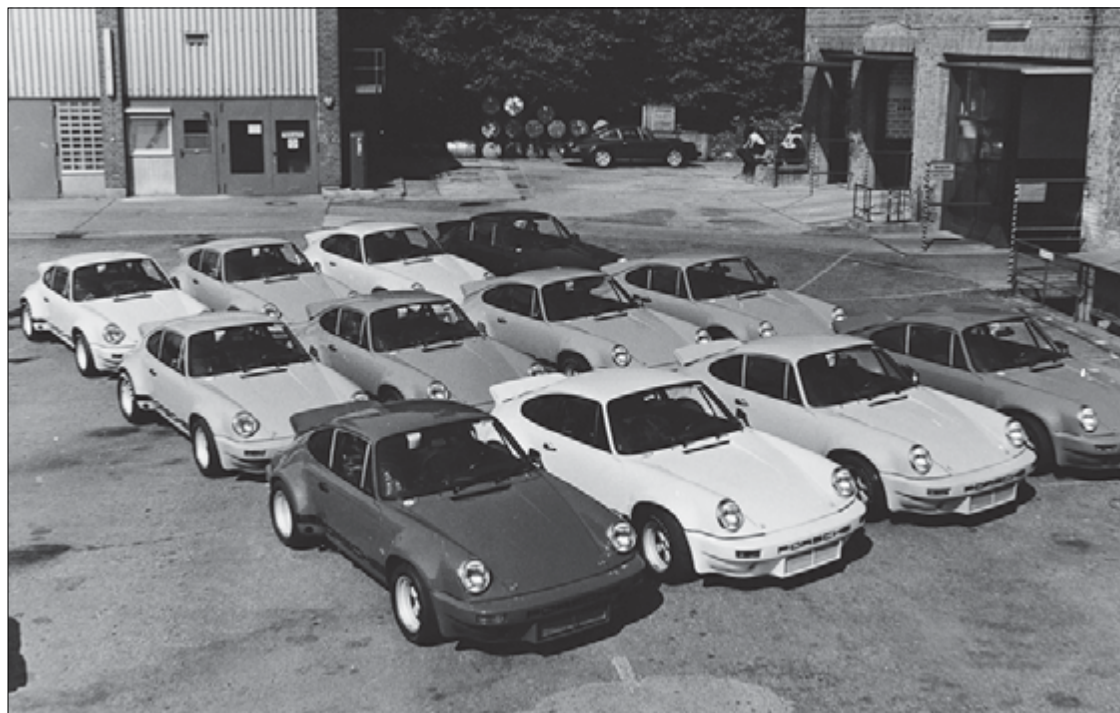
One of Porsche's greatest marketing achievements in the United States was to provide the cars for the 1974 IROC series. On the advice of race driver Mark Donohue, Roger Penske ordered fifteen Carreras to use for the 1974 International Race of Champions. The cars were a hybrid of the RS and RSR, and were built to look more like production 911s. They had flared rear fenders and a front end similar to the RSR as well as the duck's tail deck lid. A dozen of the cars are seen here at the Porsche factory late in 1973 before being readied for shipment to the United States. (PORSCHE WERKFOTO)
