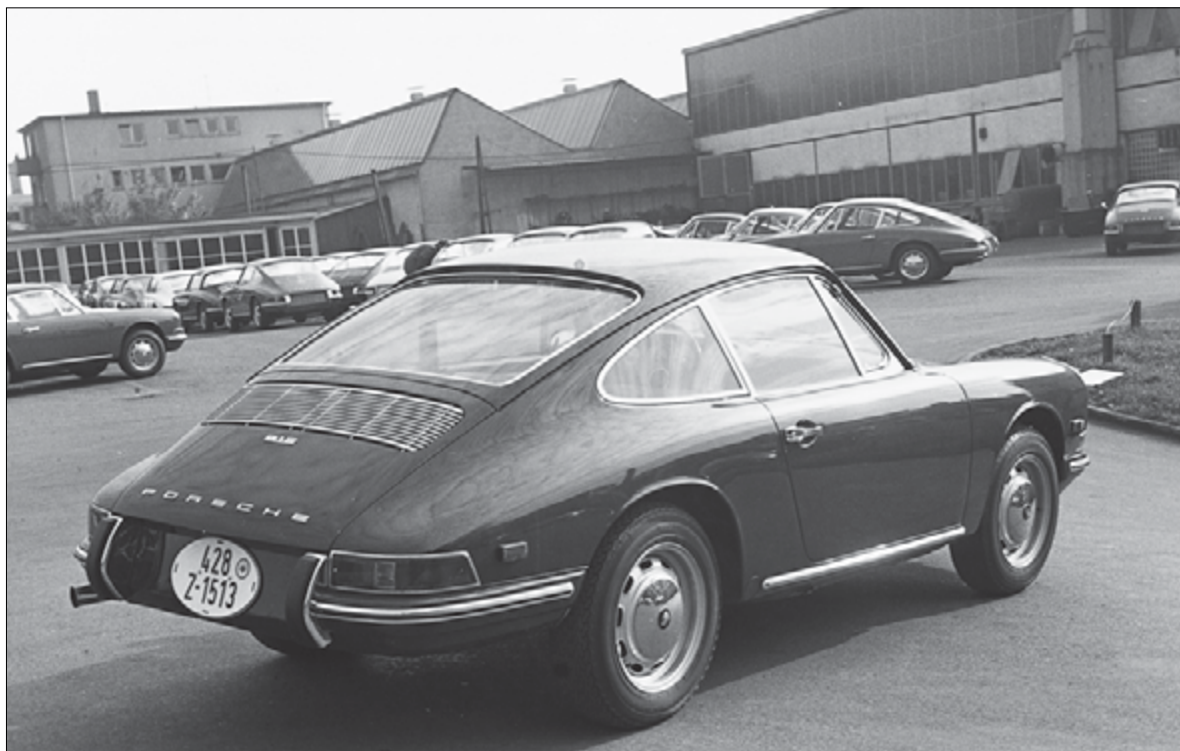
It was hard to distinguish a 912 from a 911 at a glance. Exterior lines were virtually identical, but from the rear the 912 emblem on the engine cover was an immediate tip-off. The 912 was powered by the 356C (1600SC) four-cylinder engine, making the car less potent on the road but far more affordable than the 911. In the first full year of production Porsche delivered 9,090 Type 912 models, roughly half of which were sold in the United States, beginning in June 1965, as a 1966 model. (PORSCHE WERKFOTO)
