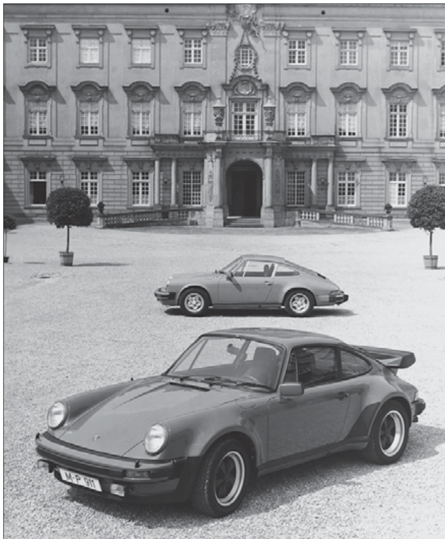
In 1978, Zuffenhausen upped the ante with the new SC 3.0 Turbo. It had a blistering 300 brake horsepower from a revised flat six with a swept volume of 2,994 cubic centimeters. (PORSCHE WERKFOTO)
