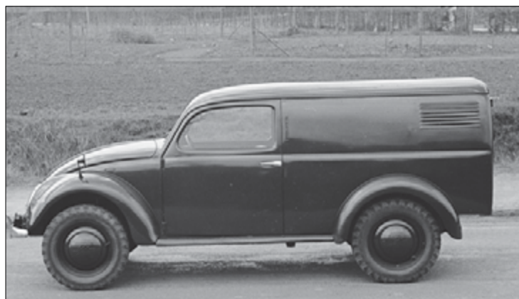
The Volkswagen was a versatile platform suitable for a variety of different bodies and uses. This was the prototype for a small truck.
