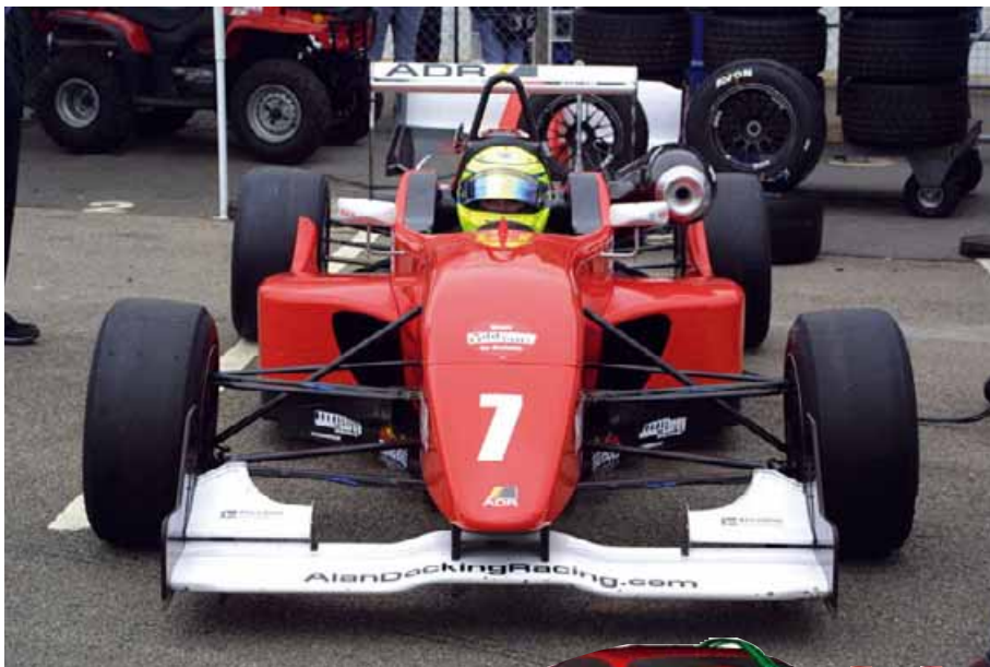
Above – figure 14: it might look like the wake from the mirror on this Dallara F305 could reach the airbox inlet, however, it was tested and does not
