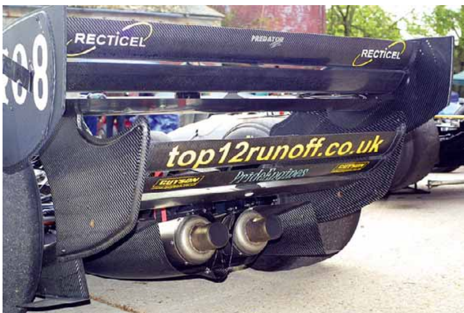
The diffuser tunnels at the back of the car integrate aerodynamically with the rear wing assembly
