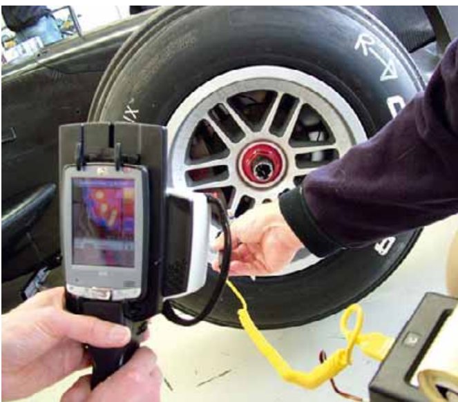
Colours can be adjusted to suit the user and the amount of colour change to temperature can also be adjusted. Racecar found the default setting to be the best
