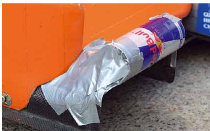
Figure 12: a less sophisticated attempt at adding a radius to an underbody inlet...
