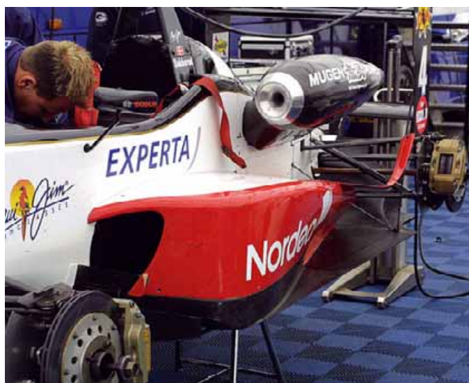
Figure 10: this Dallara F305 demonstrates nicely rounded duct inlets, and a taped-over radiator duct...
