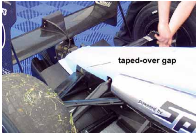
Figure 7: thin tape over gaps in bodywork can help reduce drag
