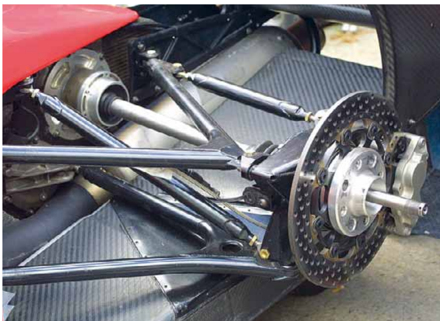
Top: front suspension uses unequal length wishbones; middle: pullrod front monoshock enabled a very low line chassis; below: rear suspension is also conventional design while rear brakes use motorbike calipers
