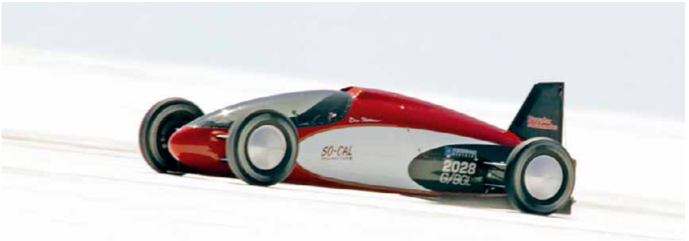
The Ecotec Lakester - a stroke of marketing genius and a class record holder at Bonneville, having reached a best of 189mph with stock 2.0-litre SC Ecotec power
