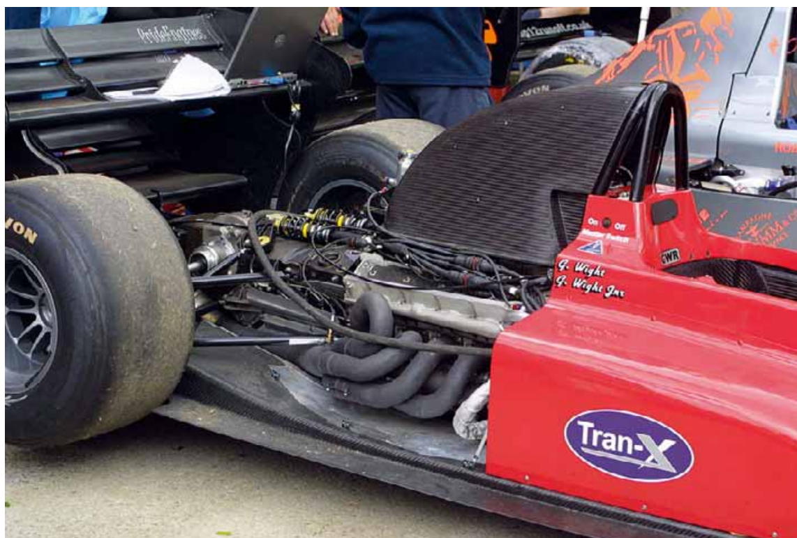
The Predator's ex-Arrows Hart V10 powertrain – longer but with more forward weight distribution than the competition
