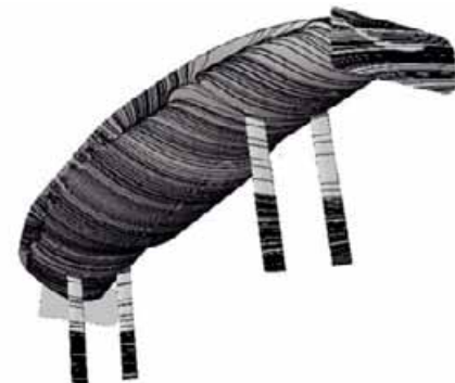
Figure 16: a modified mounting design created less disturbance to the airflow (Advantage CFD)
