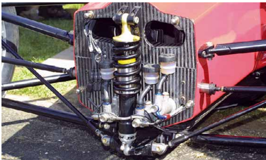
Top: front suspension uses unequal length wishbones; middle: pullrod front monoshock enabled a very low line chassis; below: rear suspension is also conventional design while rear brakes use motorbike calipers
