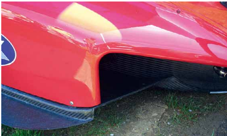
Sidepod and underbody inlets – designed so that airflow under the car can never be choked off
