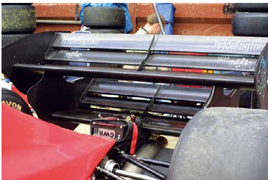
Complex twin tier rear wing assembly. The lower tier does not extend into the wake of the rear wheels
